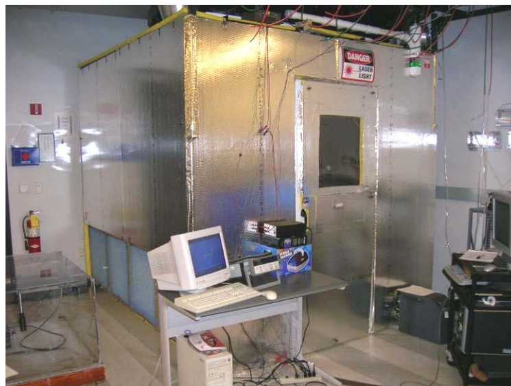
Figure 2.9: Operating Room Simulator After the Addition of Glass Fiber Insulating Panels
