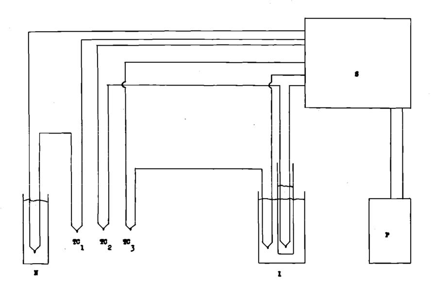
jacket, the liquid in the reservoir, and the wall of the reservoir. All the thermocouples were made of No. 34 copper and No. 32 Constantan wire.
