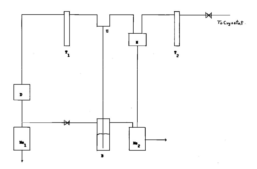
to the sample container was the primary flowmeter. These were the measurements used in determining the heat transmission. This flowmeter and its connections etc. were considered the primary flowmeter system. A diagram of the primary flowmeter system is shown in Figure 7. The system was arranged in such a manner that an accumulative meter and an instantaneous meter could be operated in series at any time desired.
