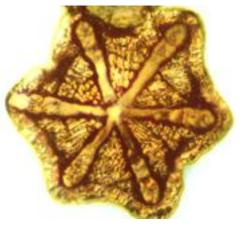
optical microscope image shows a 150micron crystal grown from 1.7 nanometer gold nanocrystals. <u>(200-dpi JPEG version - 248k)</u>
