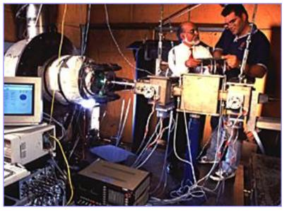
GTRI researchers have developed a unique facility to measure sound absorption properties.
