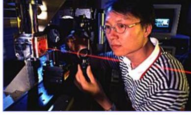
A GTRI researcher performs spectroscopic studies on new phosphors for advanced flat panel displays.
