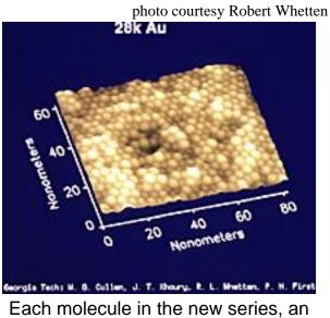
Each molecule in the new series, an array of which is shown here via scanning tunneling microscope (STM), has a compact, crystalline gold core. A shell of tightly packed hydrocarbon chains surrounds the core and is linked to it via sulfur atoms. (200-dpi JPEG version - 150k)
