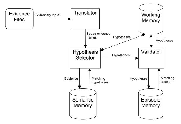
Figure 1: Architecture of Spade
