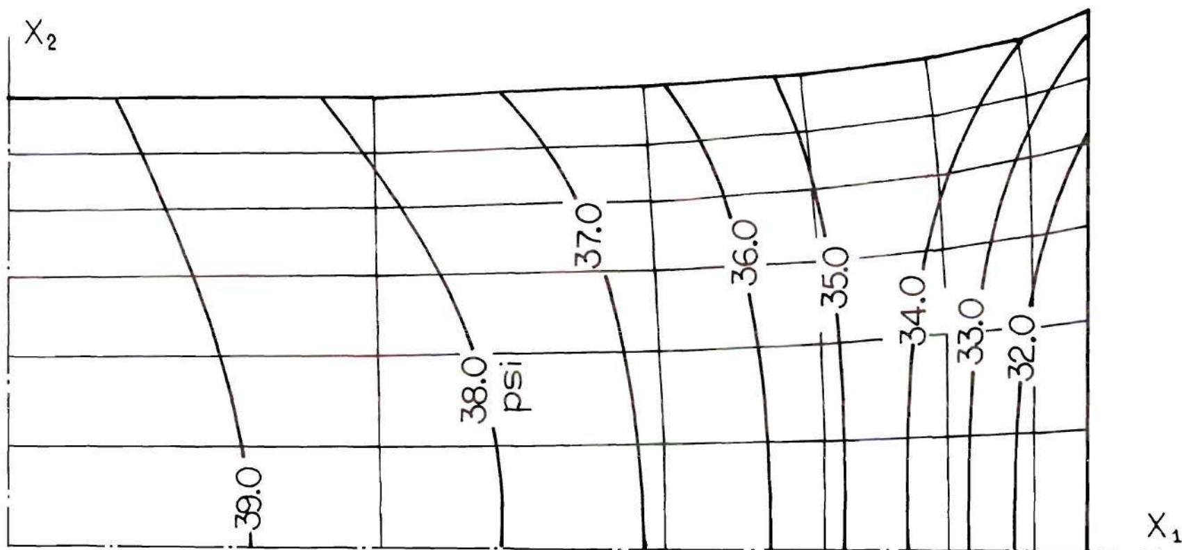
Fig. 12 Contours of Axial Component of Cauchy Stress \tau_{11} at \lambda = 2.0
