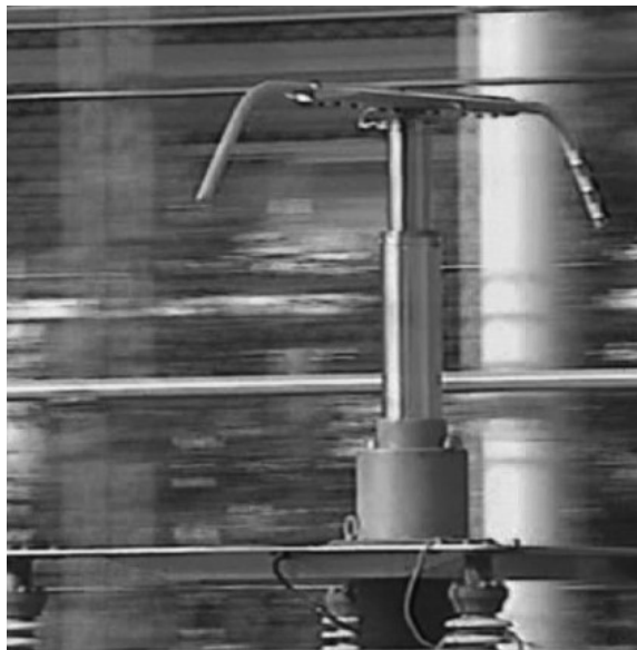
Figure 1.3: An example of a train’s pantograph: the completed “Winggraph” design solution for the Shinkansen Train example case. Adapted from [100]
