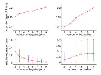
Figure 12: Average execution time and relative estimation error per operation for varying maximum hop radius and number of objects. Default parameter setting: maximum hop radius 6, number of target objects 5.
