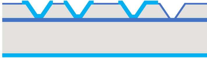
Figure A.5: Thick LPCVD TEOS deposition, patterning, and thin sacrificial thermal oxide formation.
