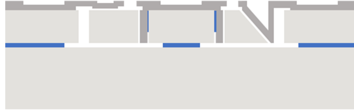
Figure A.11: Cross-sectional view of released device wafer with nano-gap vertical, horizontal, and slanted polysilicon electrodes.
