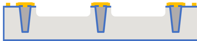
Figure A.12: Pre-bonding preparation of the capping wafer.
