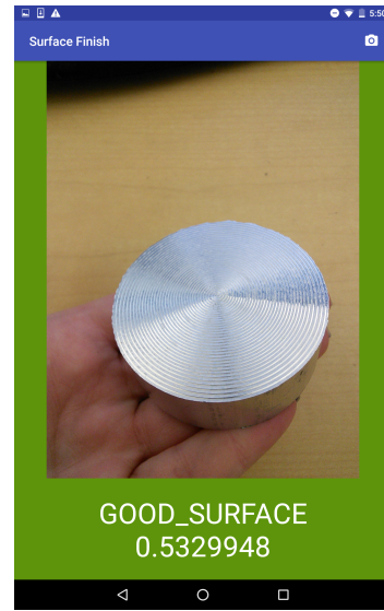
Figure 6.12: Bad surface finish parts misclassified under bright light
