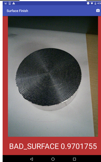
Figure 6.10: Bad surface finish detected under different lighting conditions
