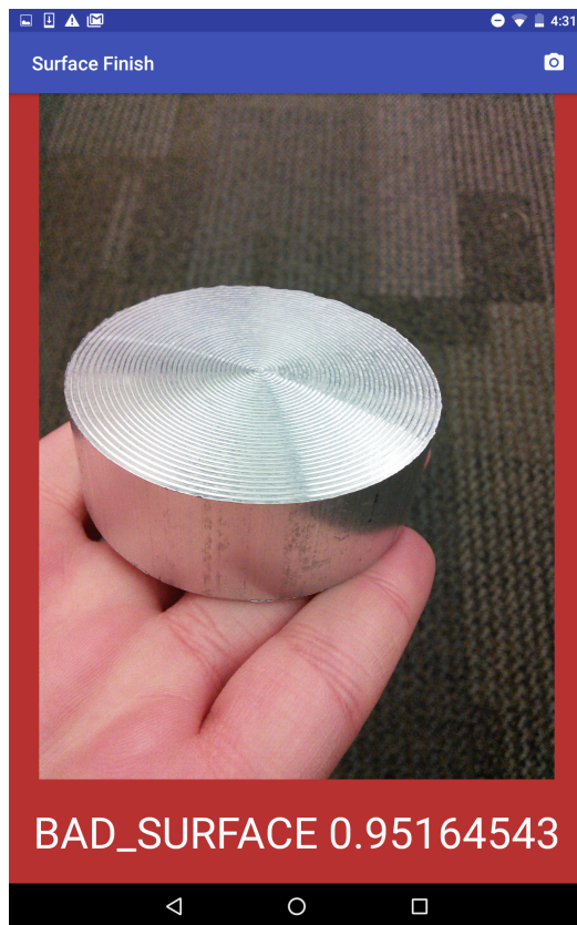
Figure 6.8: Bad surface finish detected from different angles
