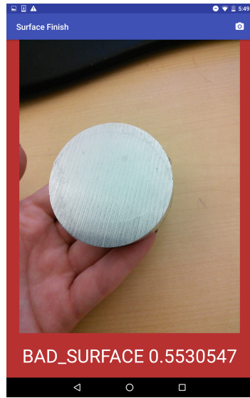
Figure 6.12: Bad surface finish parts misclassified under bright light
