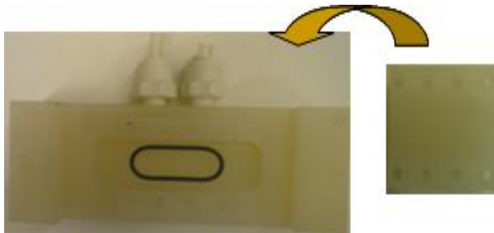
Figure 73 HF compatible cell for FTIR studies
