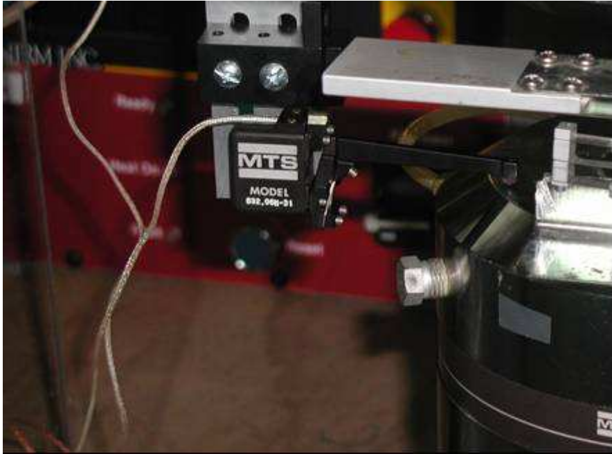
Figure 3.9. Picture of the one arm bandit applied to the low cycle fatigue setup, which uses a lever that rests on the actuator to measure actuator displacement.
