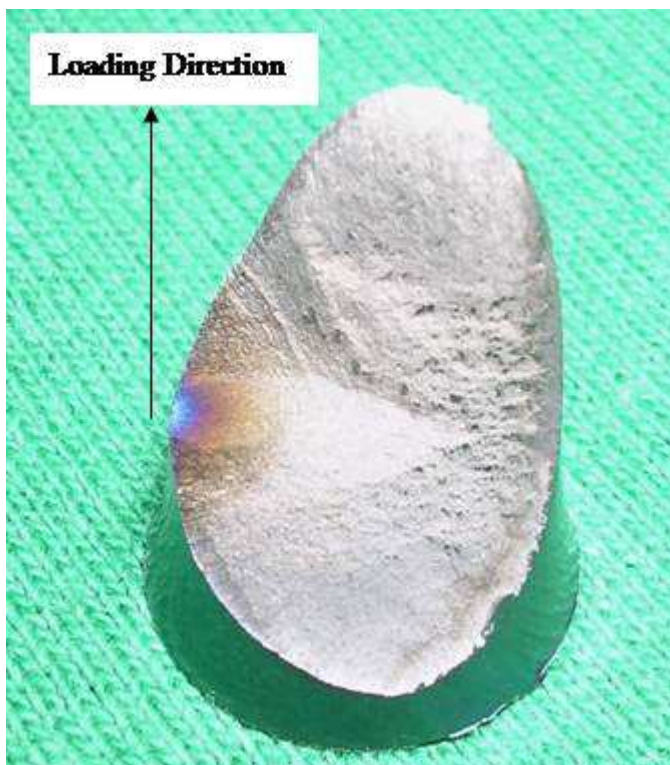
Figure 4.42. Fatigue fracture surface from a specimen tested with a strain range of 0.66% at 650°C.
