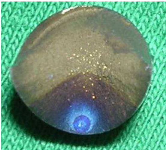
Figure 4.18. Low magnification image of the low cycle fatigue fracture surface from P 222 tested at \Delta\epsilon=0.79\% and 650^{\circ}\text{C} . The oxidation pattern outlines a subsurface crack initiation site.
