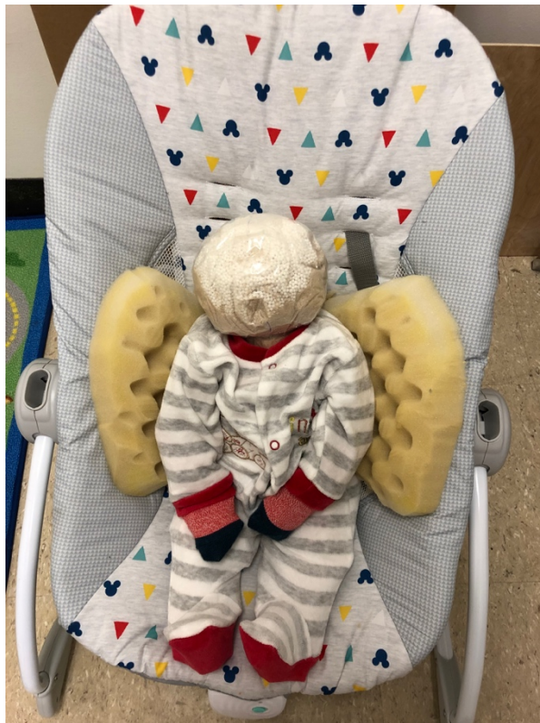
Figure 34. Foam postural support with manikin
