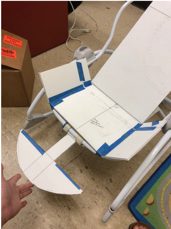
Figure 39. Foldable kickstand concept
