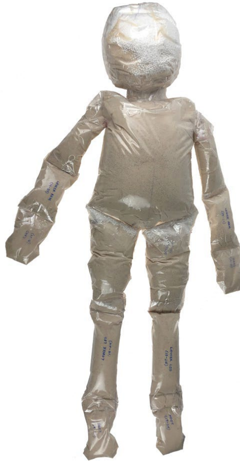
Figure 20 & 21. Completed manikins- note polystyrene beads in legs and head
