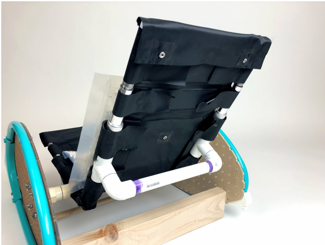
Figure 43. Detail of back – telescoping tubes visible
