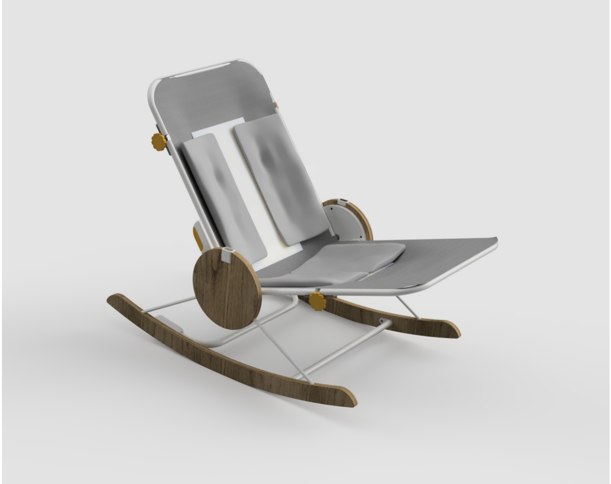
Figure 49. Rocker without slip cover; nylon hammock, plastic sheets, and EPP bladders visible
