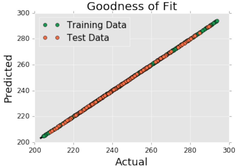
Figure 20: Goodness-of-Fit plot for effective stiffness C_{xx} for the homogenization model.
