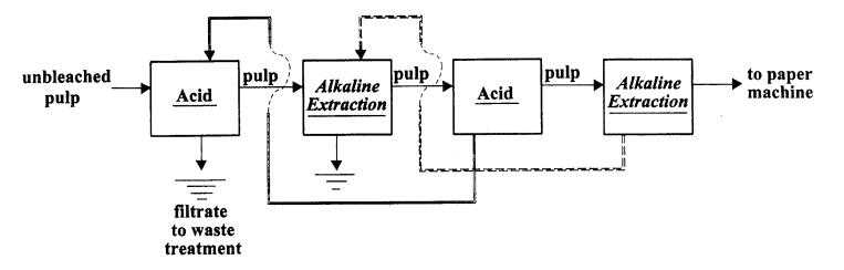
Fig. 2 Accumulation of calcium in a three-stage, laboratory simulation of water recycle in a bleach plant.
