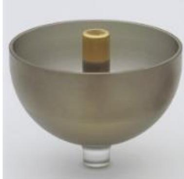
**Figure 1.8: Fused quartz hemispherical shell resonator (HSR)**
