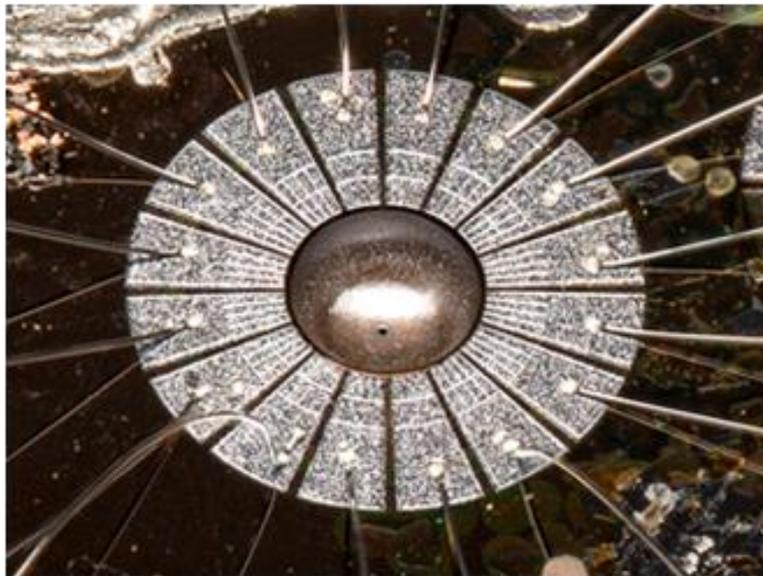
**Figure 7.3: A polysilicon  $\mu$ HRG with all 16 electrodes bonded to the interface PCB**
