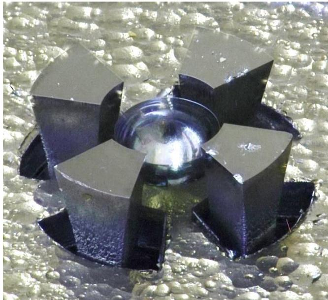
**Figure 3.7: Microscope image of assembled  $\mu$ HSR**
