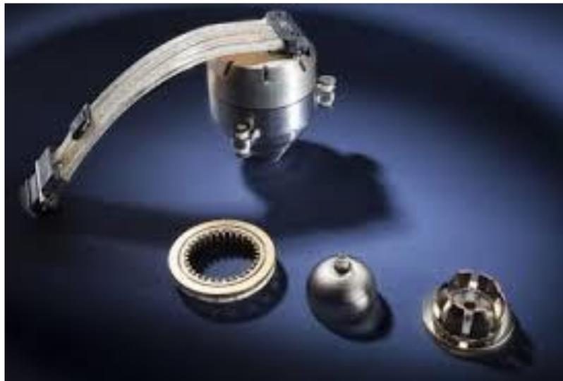
**Figure 1.7: Hemispherical Resonator Gyroscope (HRG) Assembly
