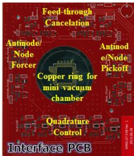
Figure 7.1: Layout of interface PCB
