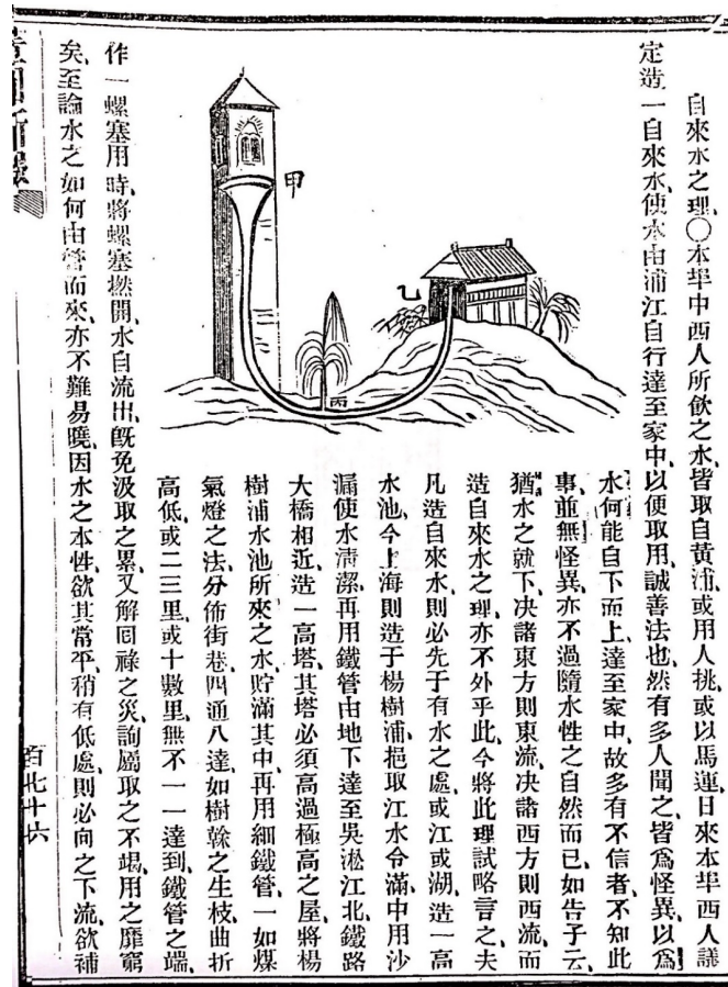
Figure 16 – Illustration of the working of water supply. The Chinese explanation was to educate the Chinese on the matter. Source: “Zilaishui zhi li (futu)”, 1881.
