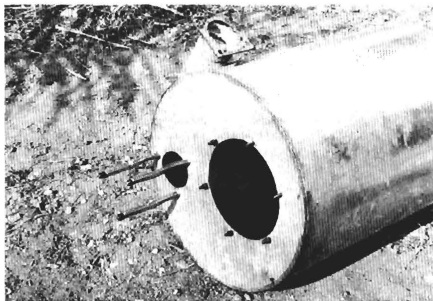
Figure 6. View of the condenser which shows where the cyclone (large hole) and pressure relief port (small hole) are located
