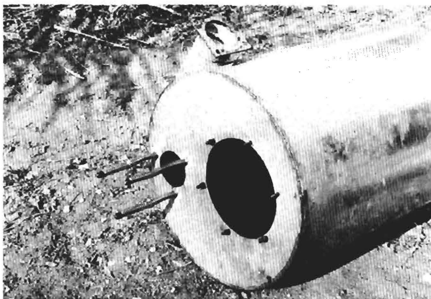
Figure 8. View of the condenser which shows where the cyclone (large hole) and pressure relief port (small hole) are located
