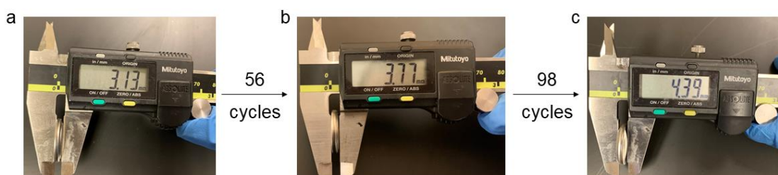
Figure 4.2 - Thickness measurement of a Ni-Zn SS coin cell over cycling with zinc foil as the anode.
