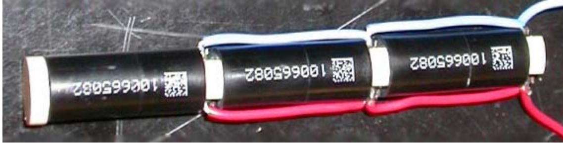
Figure 4.3.2: Picture of three bonded EPCOS stacks
