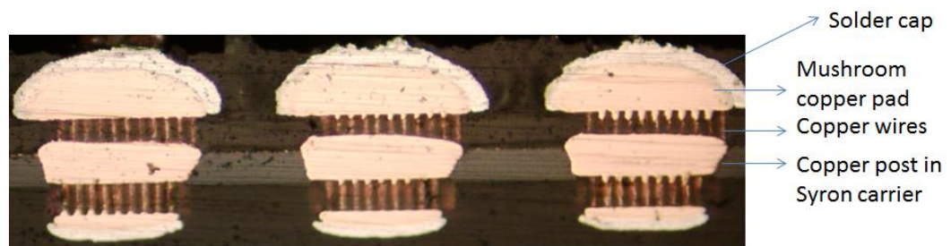
Figure 2.18: Cross section of MWA interconnections.
