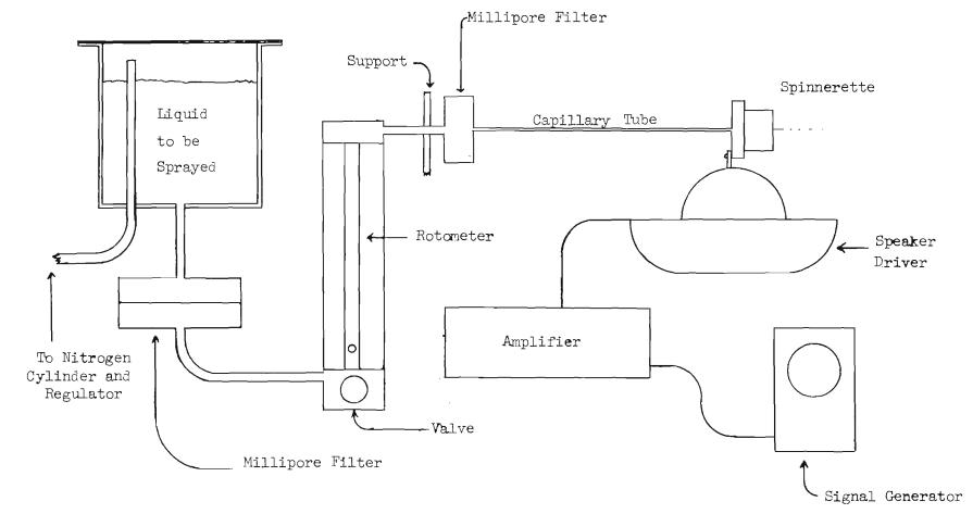
Figure 1. Audio Atomizer Apparatus
