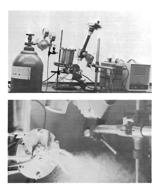
Figure 10. Photographs of the Ultrasonic Atomizer with Multiple Orifices. The top photograph is an overall view and the buttom shows a closeup of the orifice while a cloud is being generated. orifices of this study at various pressures. All the jets produced were found to have the same dimension as the orifice within the accuracy of the measurements. In other words, the coefficient of contraction was unity for all the situations investigated. A typical jet stream is shown in Figure 3.
