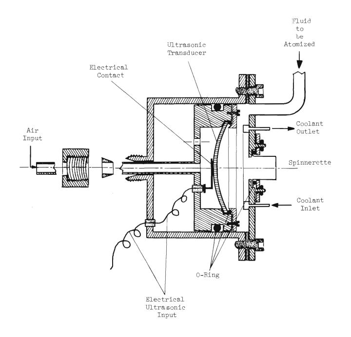
Figure 9. Ultrasonic Atomizer
