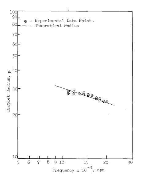
Figure 8. Droplet Radius as a Function of Vibration Frequency as Produced with Dow Corning Silicone Oil (viscosity, 1 centistoke) Flowing Through a 20-µ Diameter Orifice at a Rate of 0.138 cm<sup>3</sup>/min. arrangement.
