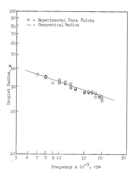
Figure 6. Droplet Radius as a Function of Vibration Frequency as Produced with Water Flowing Through a  $20{-}\mu$  Diameter Orifice at a Rate of 0.17  $\rm cm^3/min.$
