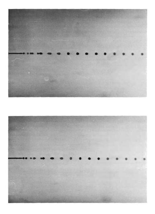
Figure 3. Photographs Showing the Absence of Contraction in Jets but Showing Droplet Coagulation.
