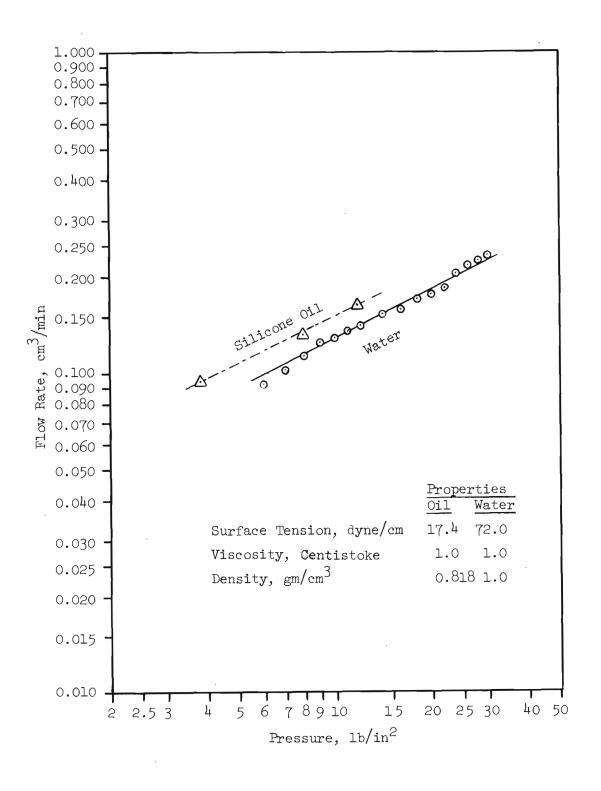
Figure 11. Flow Rate as a Function of Pressure for a 20µ Diameter Orifice.
