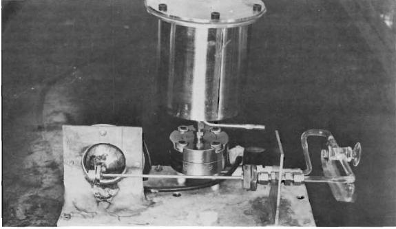
Figure 2. Photographs of the Audio Atomizer Employing a Single Orifice. The top photograph is an overall view and the bottom shows a closeup of the orifice holder and flow meter.
