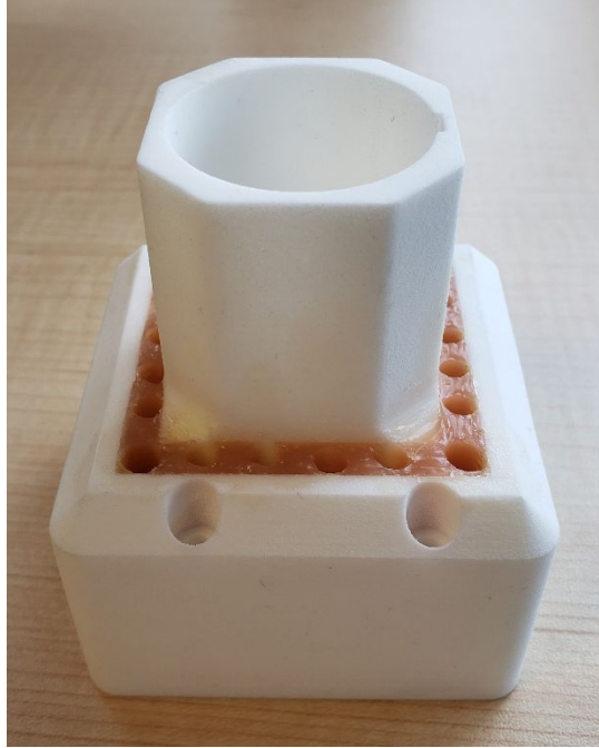
Figure 17: 3D Printed Flexible Coupler
