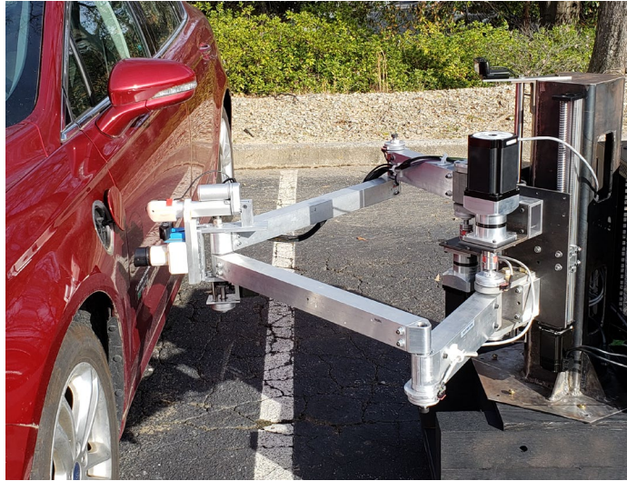
Figure 11: Parallel Arm SCARA Robot for autonomous EV charging
