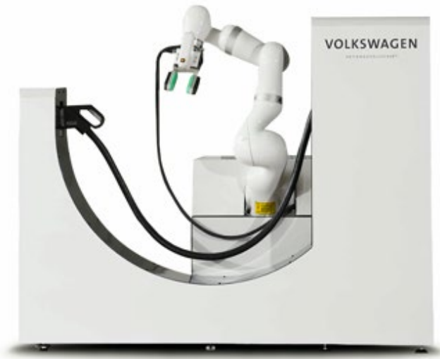
Figure 3: Volkswagen e-smartConnect Automated EV Charging System
