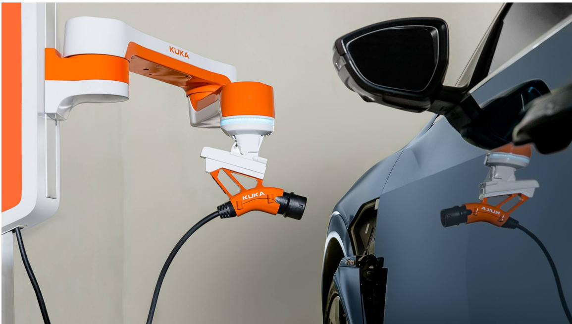
Figure 4: Kuka Carla_connect Automated EV Charging System
