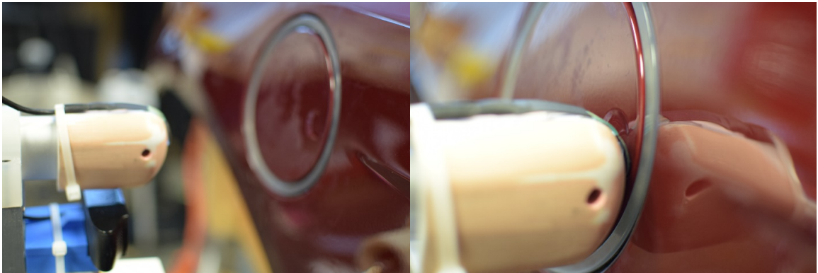
Figure 19: Alignment and “Passing” contact between Extruder and Detent
