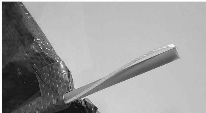
Figure 8: Photo of a commercially available threading tool, or straw, threading an earthbag hem. Source: Author 2022.
