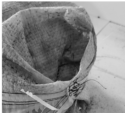
Figure 7: A schematic Corner-Stitch modification on a commercial low-duty woven polypropylene earthbag. Source: Author 2022.
