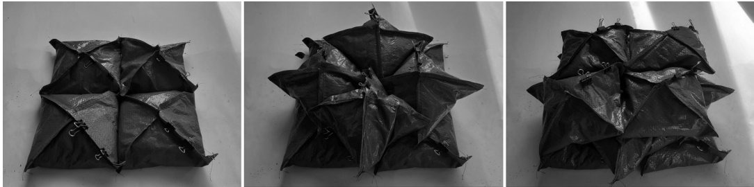
Figure 5: Gradual slippage of Surprise-Star earthbags in a 2 by 2 square alternating stack sequence (left to right). Source: Author 2022.
