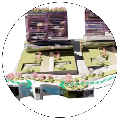
WATER RETENTION POND TO HOLD AND DISTRIBUTE WATER Max Capacity - 33,14,865 gal. (approx)
