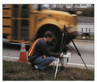
Georgia Tech researchers use remote sensing equipment at highway entrance and exit ramps to monitor vehicle emissions.
