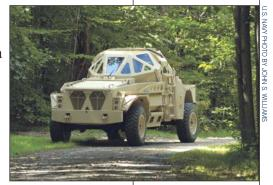
ABOVE: The ULTRA AP (Armored Patrol) vehicle is a research project funded by the Office of Naval Research and conducted by the Georgia Tech Research Institute. The vehicle features an innovative survivable crew capsule (below) that uses a new combination of armor materials, a commercial truck chassis and faceted crew capsule geometries to provide better deflection of pressure waves from blasts.
