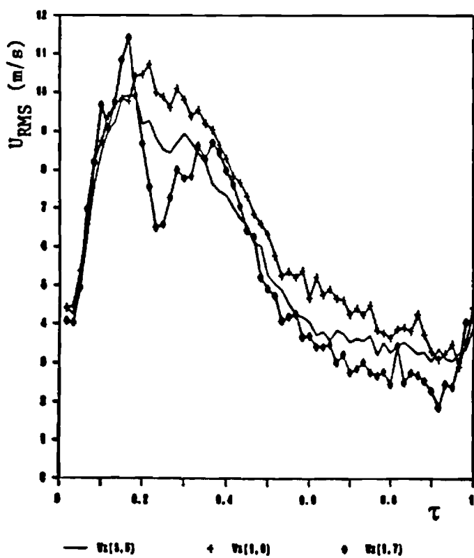
Fig. 23 Variation of the Axial Turbulence Intensity ( u_{RMS} ) with Instant During a Cycle ( \tau ) for Locations along the Line m = 3 .
