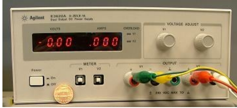
Figure 4.4: Power supply used to power the heater and the pump during testing has an uncertainty of \pm 0.25 W
