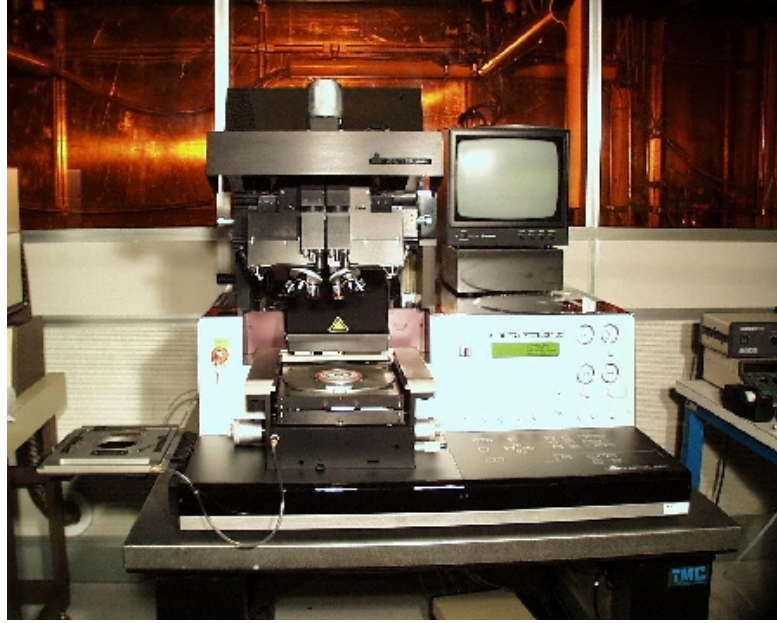
Figure 3.5: Mask alignment tool used to expose the photoresist with the mask pattern
