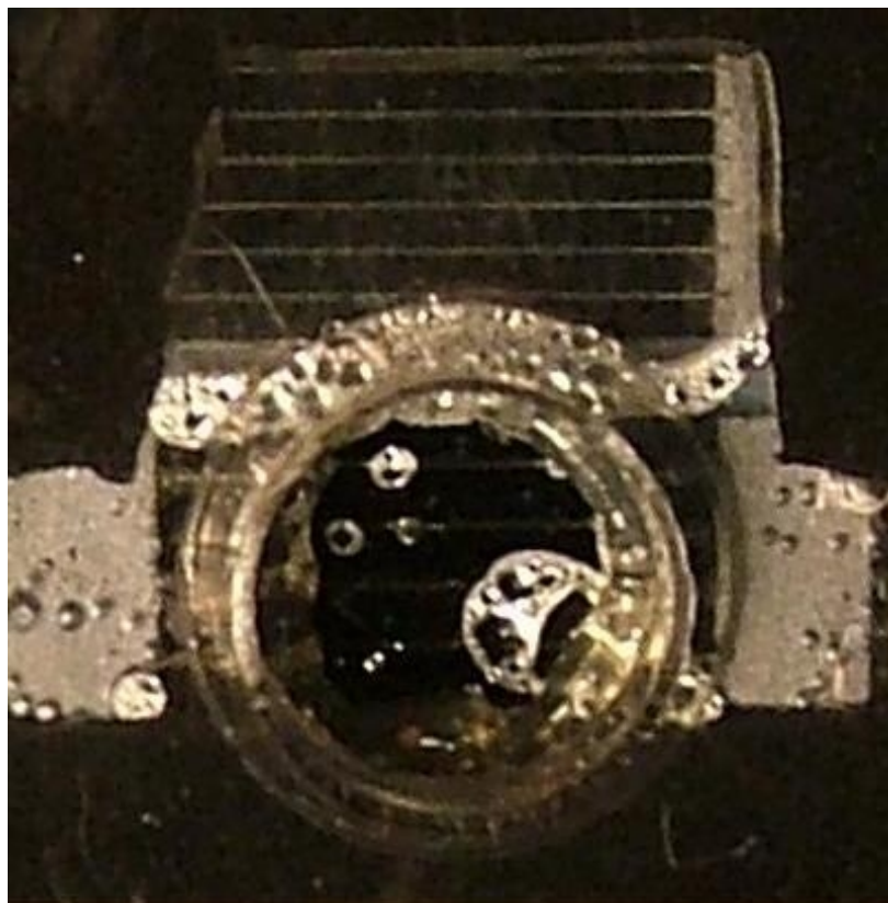
Figure 10.2: A photograph of bubbles in the device during testing, the water flow is from left to right. The circle in the center of the photo is the 9.5 mm sapphire window.
