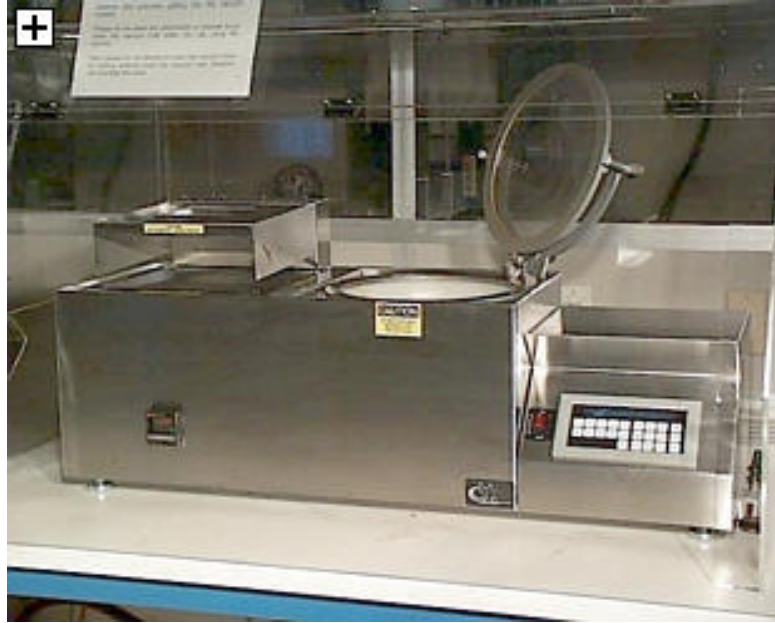
Figure 3.4: Photoresist spinner and hot plate used to spin a thin layer of photoresist on each wafer and dry the wafer after deposition
