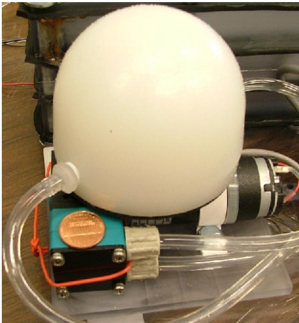
Figure 6.7: Diaphragm pump and pulse dampener used for device tests.
