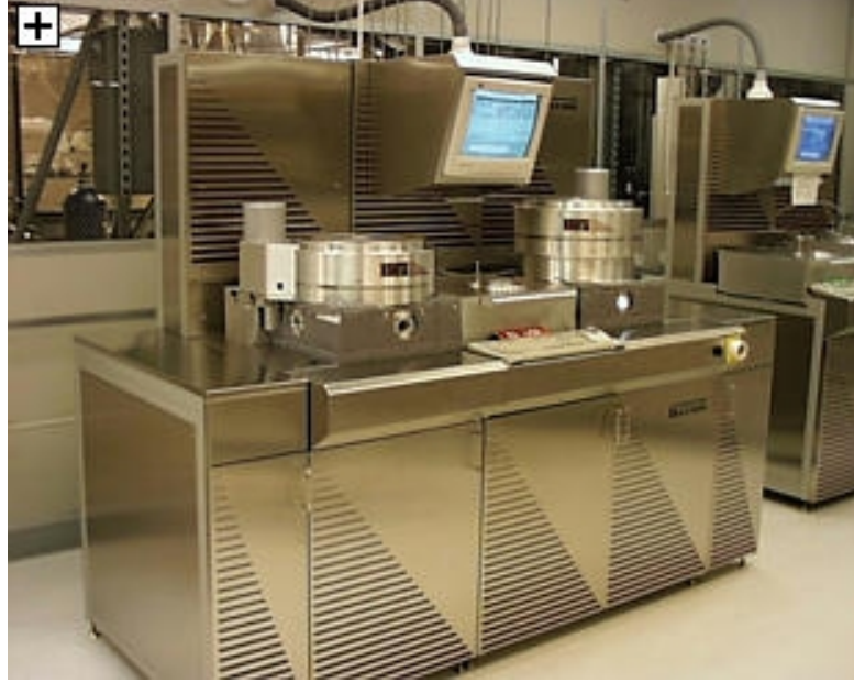
Figure 3.6: Inductively Coupled Plasma etcher used in a 2-step process to etch rectangular channels into the silicon
