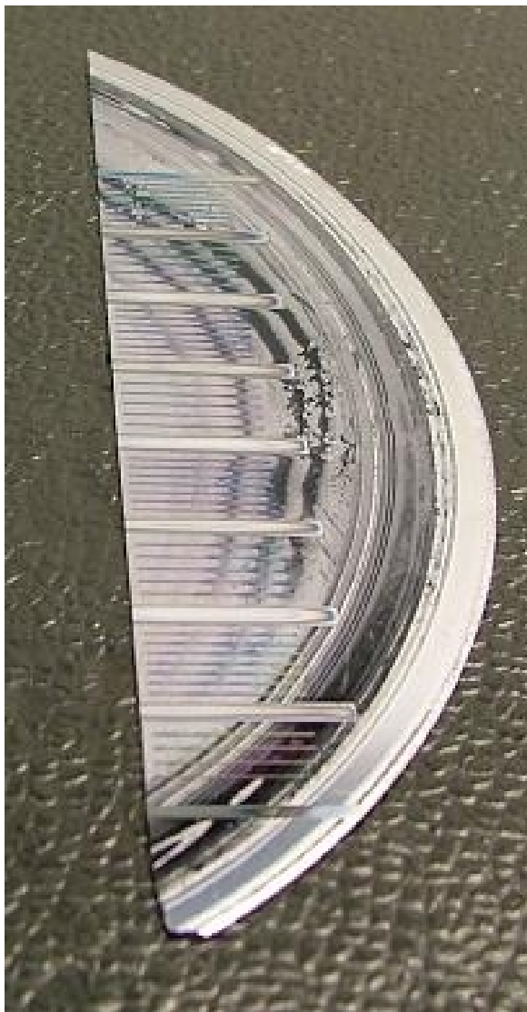
Figure 3.10: A photograph of a section of the 15.2 cm diameter wafer after the scribe and break process
