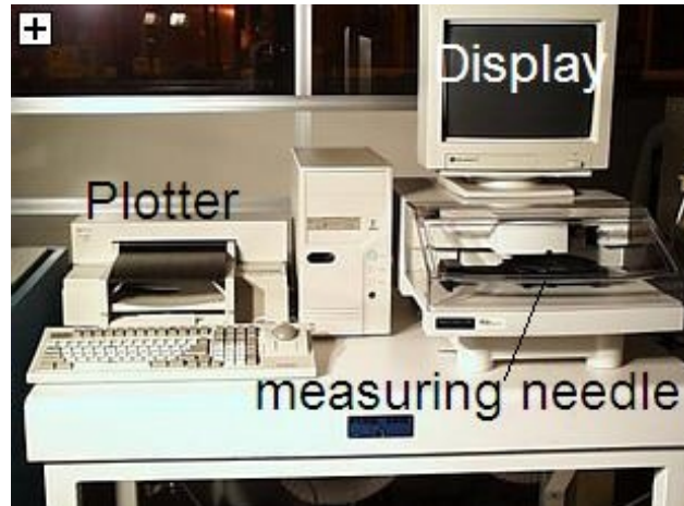
Figure 3.8: The profilometer used to determine the surface roughness of the channels
