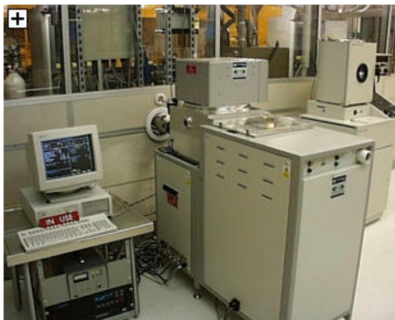
Figure 3.3: Silicon dioxide depositor used to deposit a 1\ \mu\text{m} thick layer of silicon dioxide on each wafer
