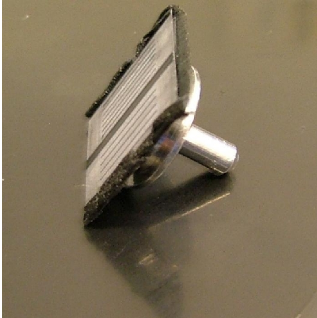
Figure 7.1: Device prepared for imaging with the SEM
