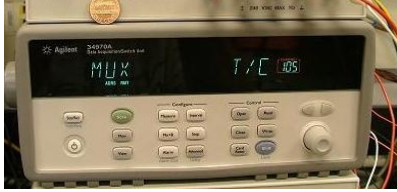
Figure 4.2: Agilent data acquisition/switch unit provides the physical connection between the thermocouples and the data acquisition software
