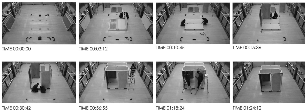
Figure 15: Full-scale assembly test of Wachsmann-based modular system. Source: Author 2018.
