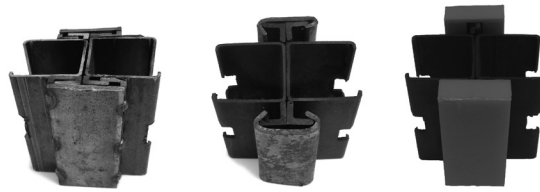
Figure 11: These three clip and node experiments explored the differences between the fabrication process for crafting the sliding node through welding, forging, and 3D printing. Source: Author 2018.
