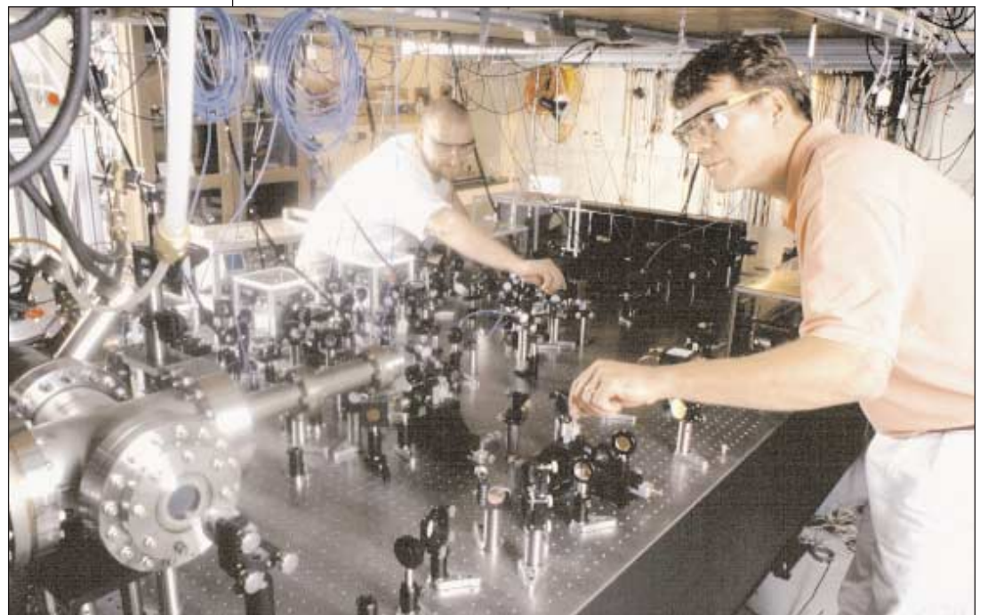
Georgia Tech researchers Michael Chapman and Murray Barrett adjust the optics of lasers used to cool and confine Bose-Einstein condensates in their lab.
