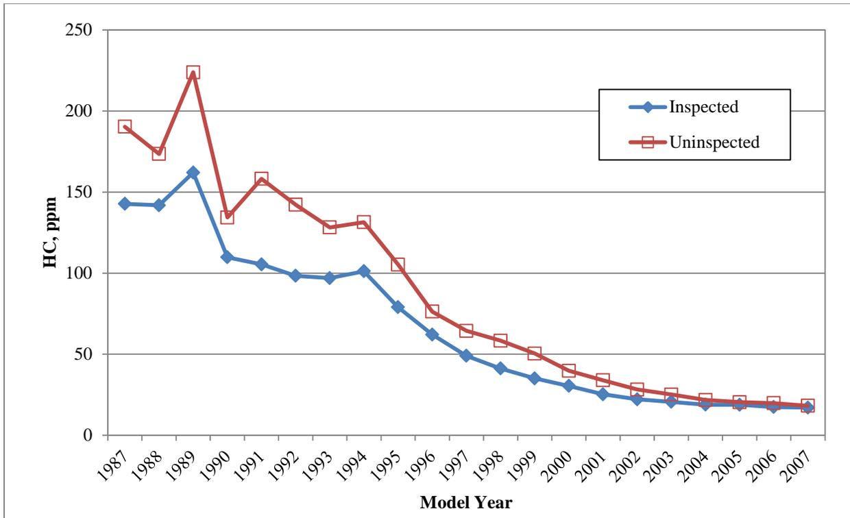
*Figure 2-3 Hydrocarbons vs. model year for inspected and uninspected fleet*
