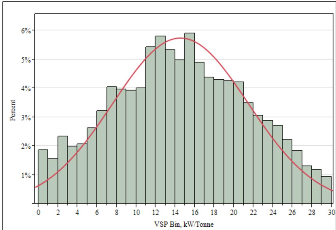
*Figure 4-21 Vehicle specific power distribution for ‘before’ repair sample for vehicles that failed the emission inspection test*
