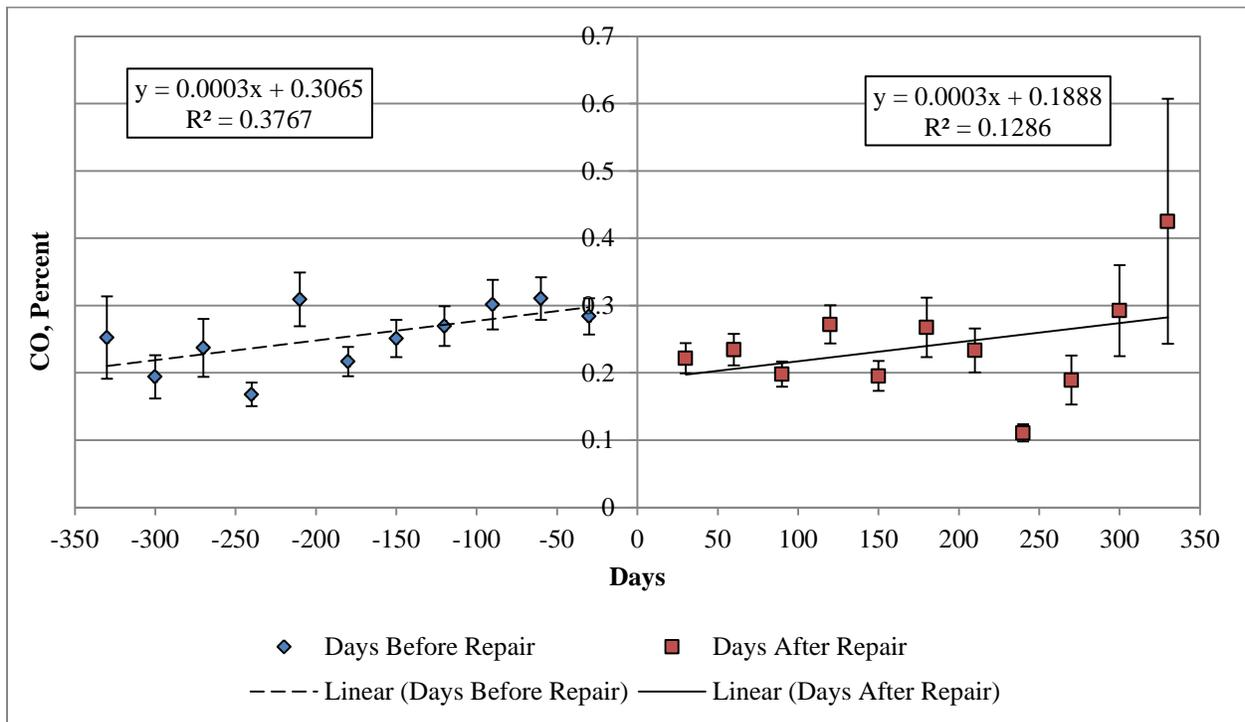
*Figure 4-35 CO measurements 'before-and-after' repair for vehicles that failed the emission inspection test*
