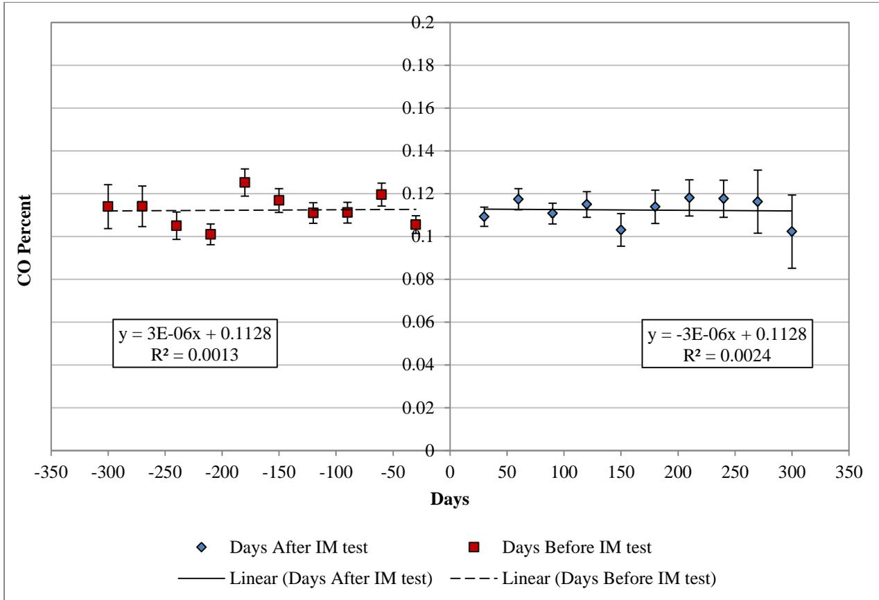
*Figure 4-15 CO Measurements days before and after emission test for vehicles that did not fail the emission inspection test*
