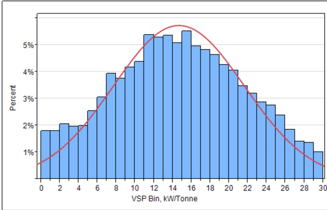
*Figure 4-20 Vehicle specific power distribution of failed-and-repaired vehicles for vehicles that failed the emission inspection test*
