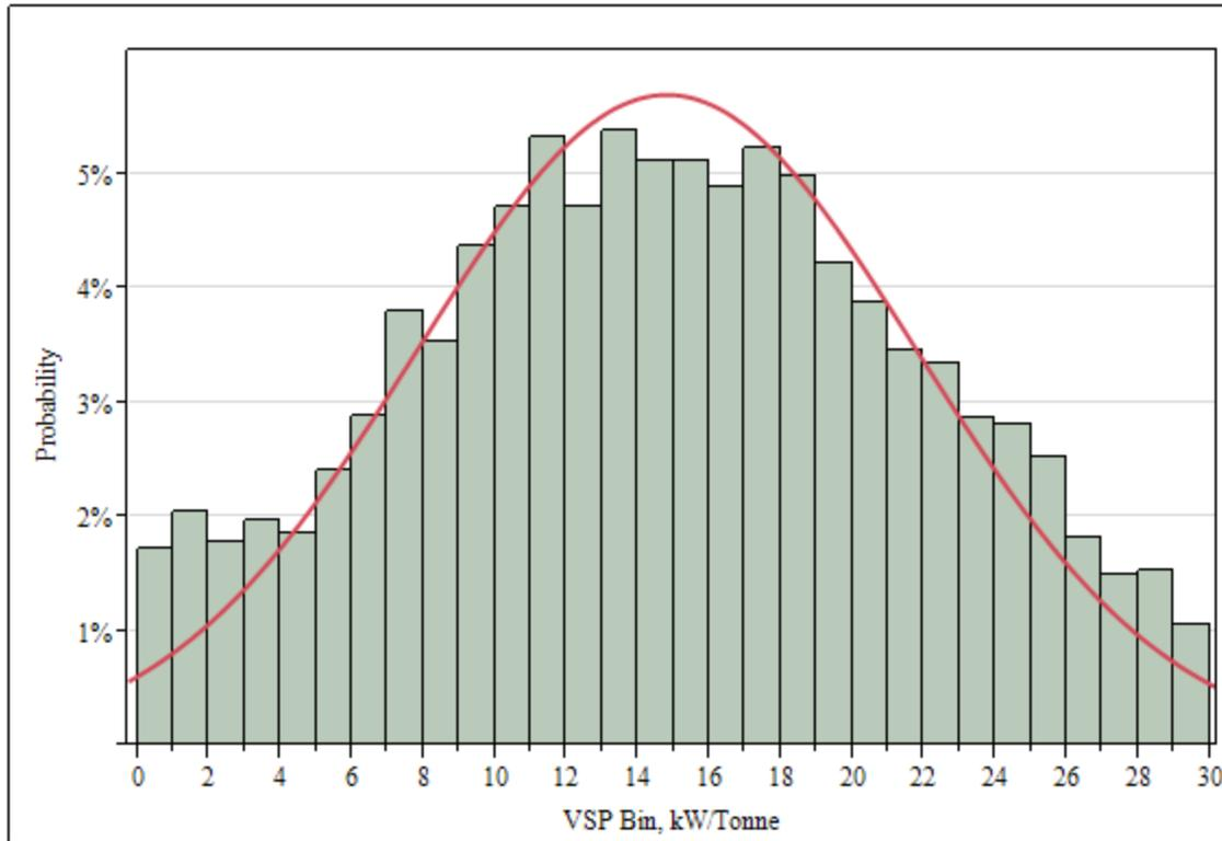
*Figure 4-22 Vehicle specific power distribution for ‘after’ repair sample for vehicles that failed the emission inspection test*
