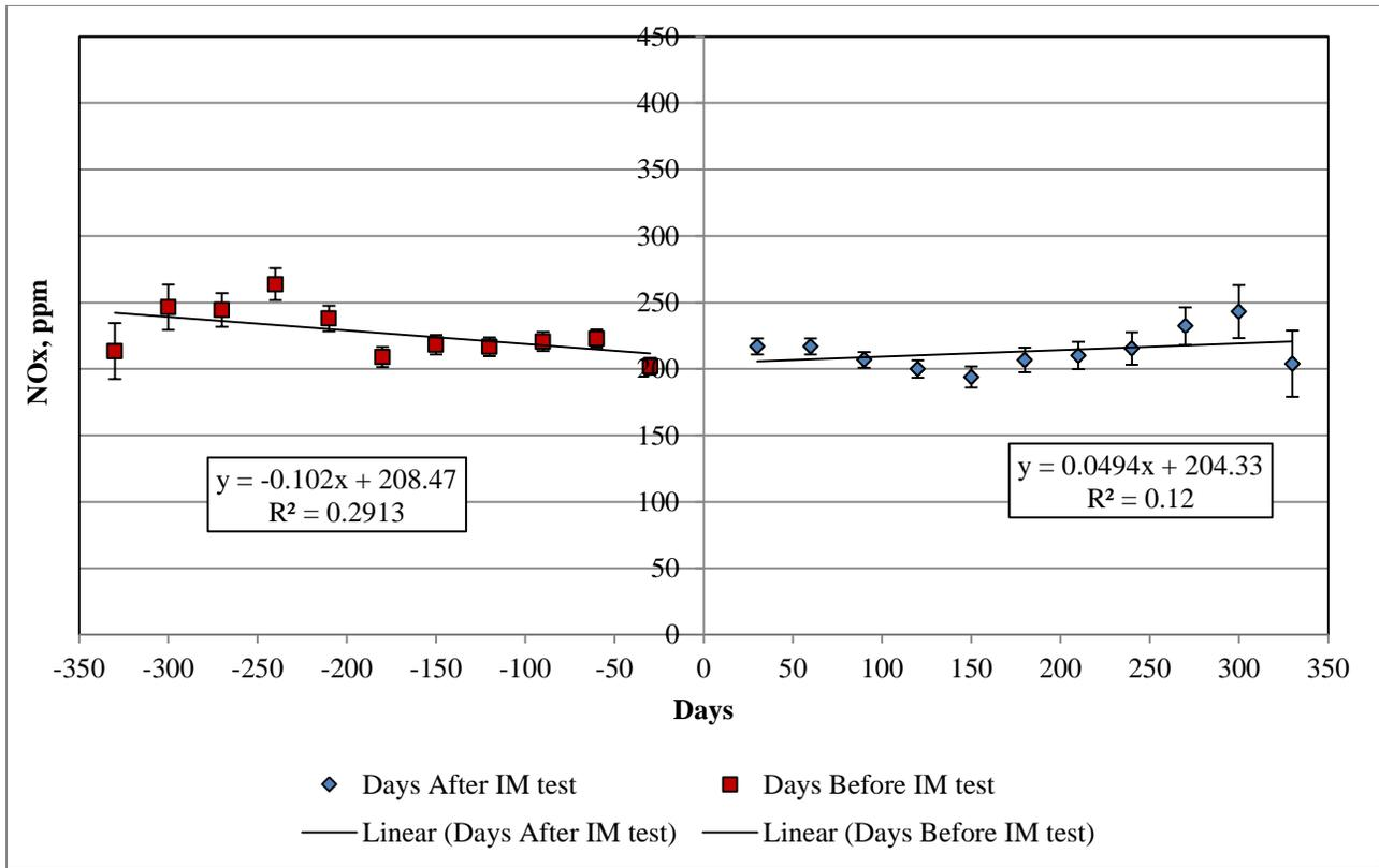
Figure 4-17 NOx days before and after emission test for vehicles that did not fail the emission inspection test
