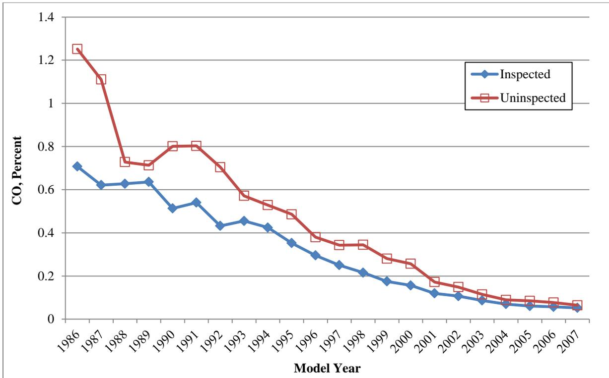
*Figure 2-2 Carbon monoxide vs. model year for inspected and uninspected fleet*
