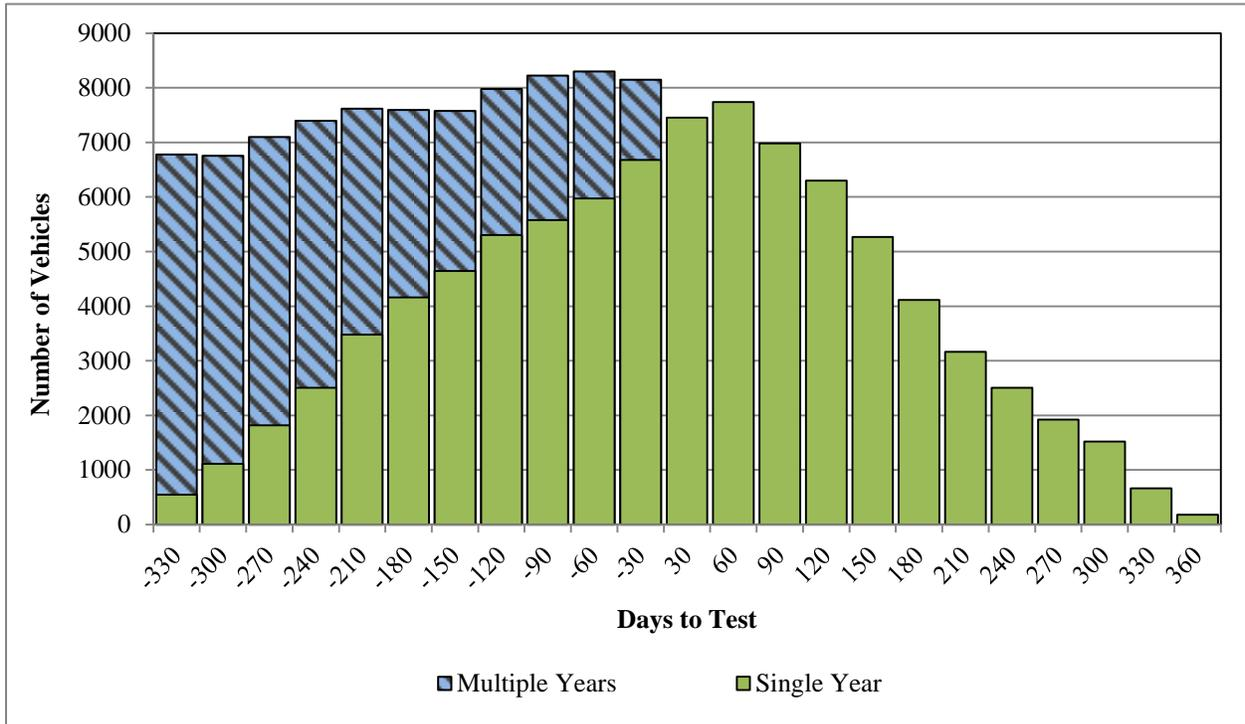
Figure 4-19 Number of vehicles in day bins: addition of multi-year emission results for the single year before and after emission test for vehicles that did not fail the emission inspection test
