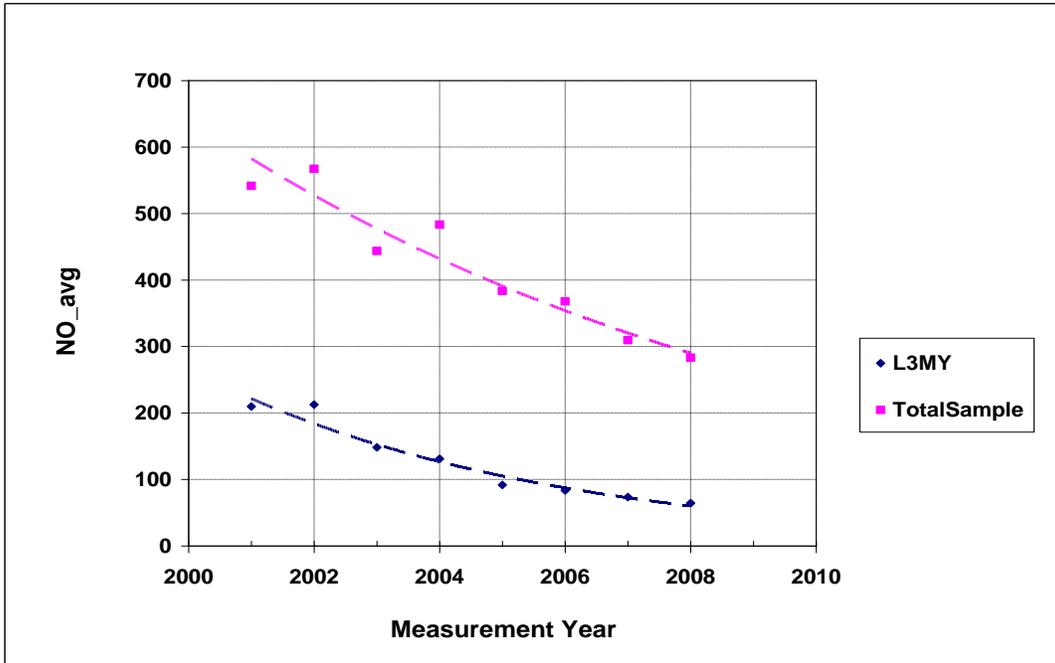
*Figure B-10 NOx average total sample and vehicles of latest three model years at different measurement years*
