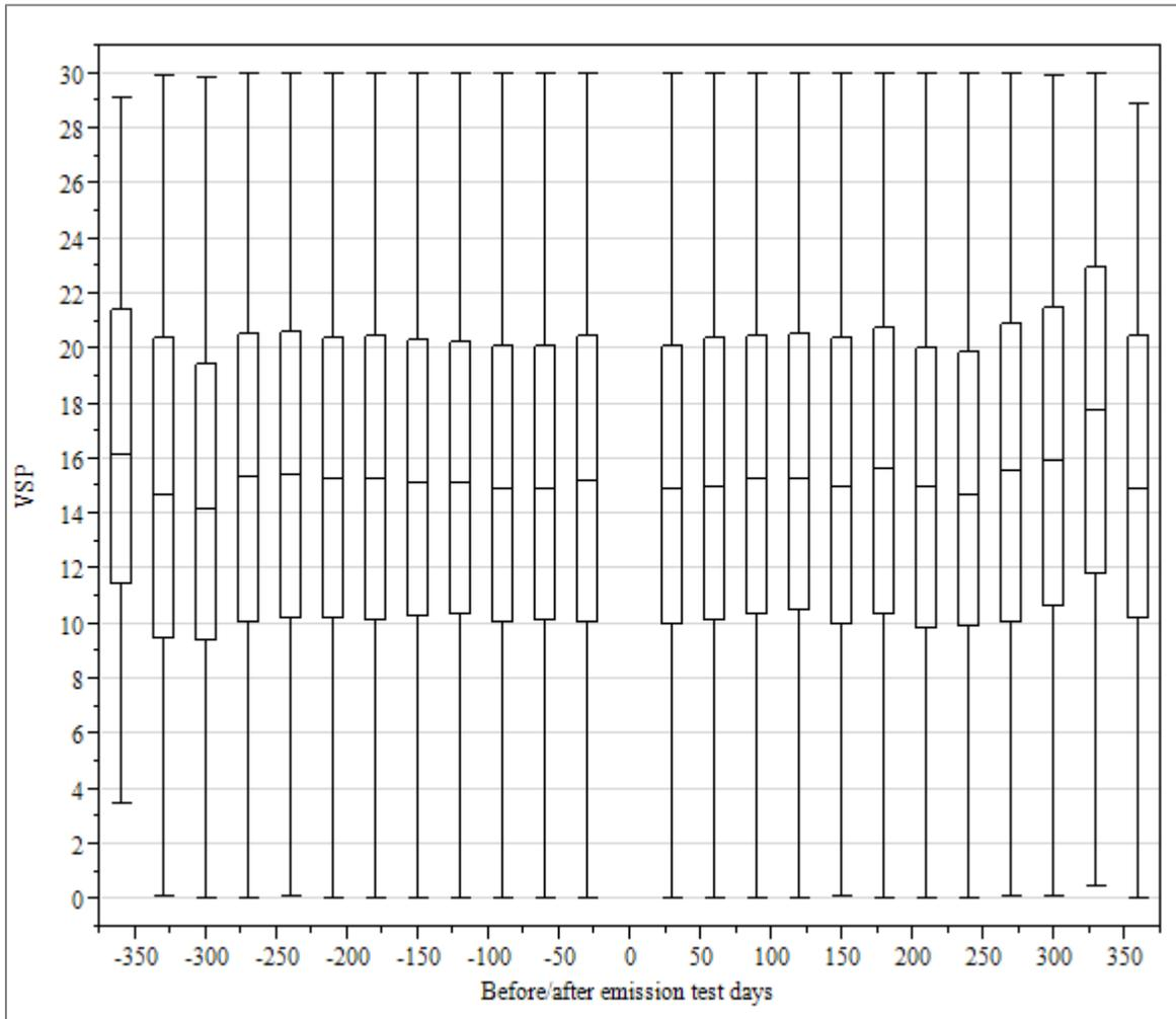
*Figure 4-12 VSP vs days before and after emission inspection test for vehicles that did not fail the emission inspection test*
