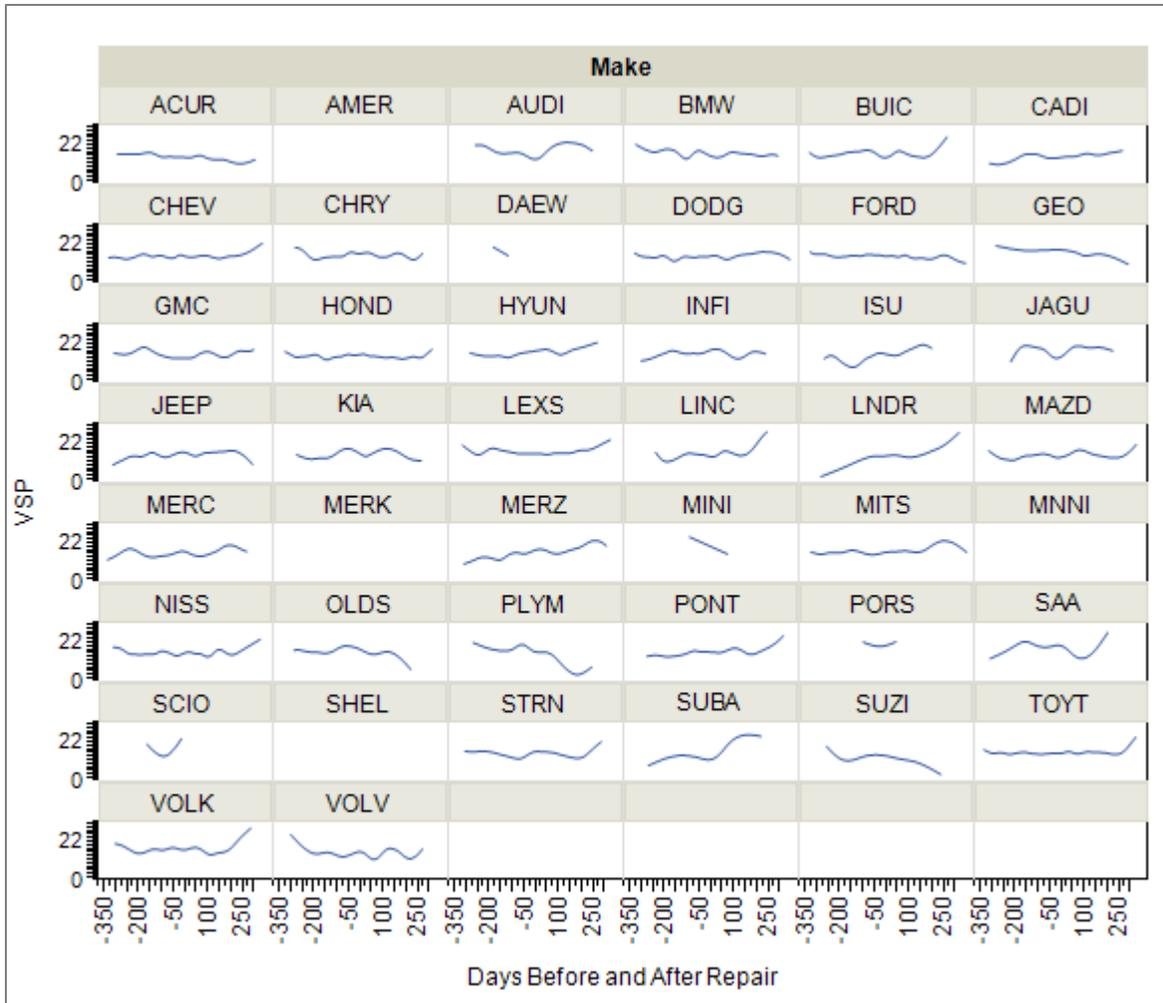
Figure A-5 Vehicle Make Vehicle Specific Power profiles for 'before' and 'after' repair sample
