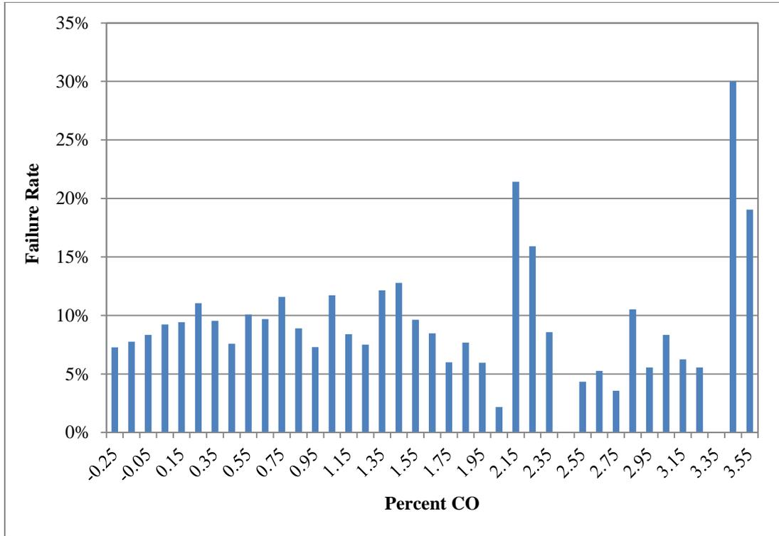
*Figure 5-3 Emission test failure rate vs vehicle emission remote sensing carbon monoxide reading*
