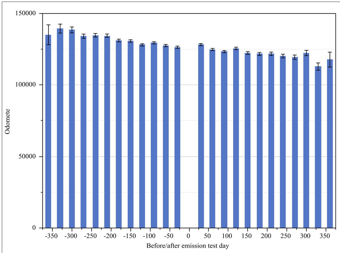
*Figure 4-14 Odometer vs days before and after emission inspection test for vehicles that did not fail the emission inspection test*
