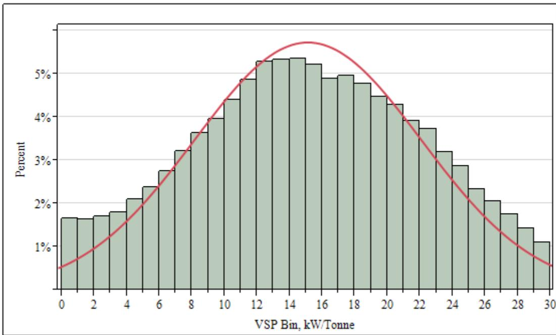
*Figure 4-2 Vehicle Specific Power distribution of ‘before’ emission test sample*
