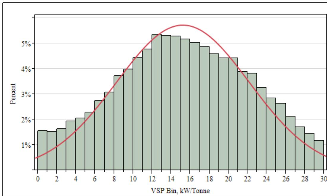
Figure 4-3 Vehicle Specific Power distribution for 'after' emission test sample
