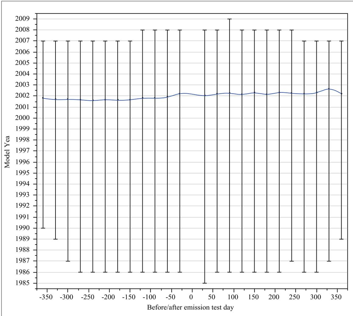
*Figure 4-13 Model year vs days before and after emission inspection test for vehicles that did not fail the emission inspection test*
