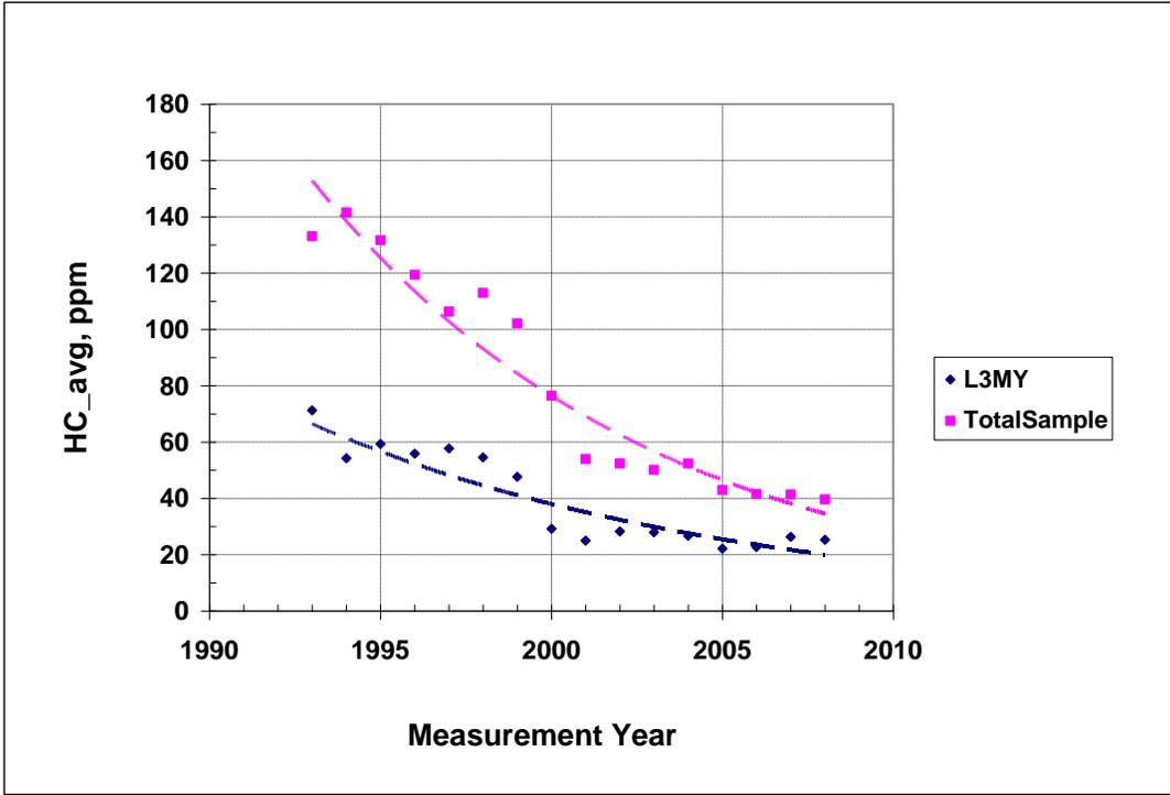
*Figure B-9 HC average years sample and vehicles of latest three model years at different measurement years*
