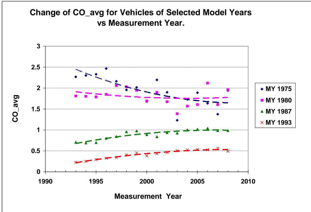
Figure B-11 Change of CO emission from vehicles of various model years by measurement year
