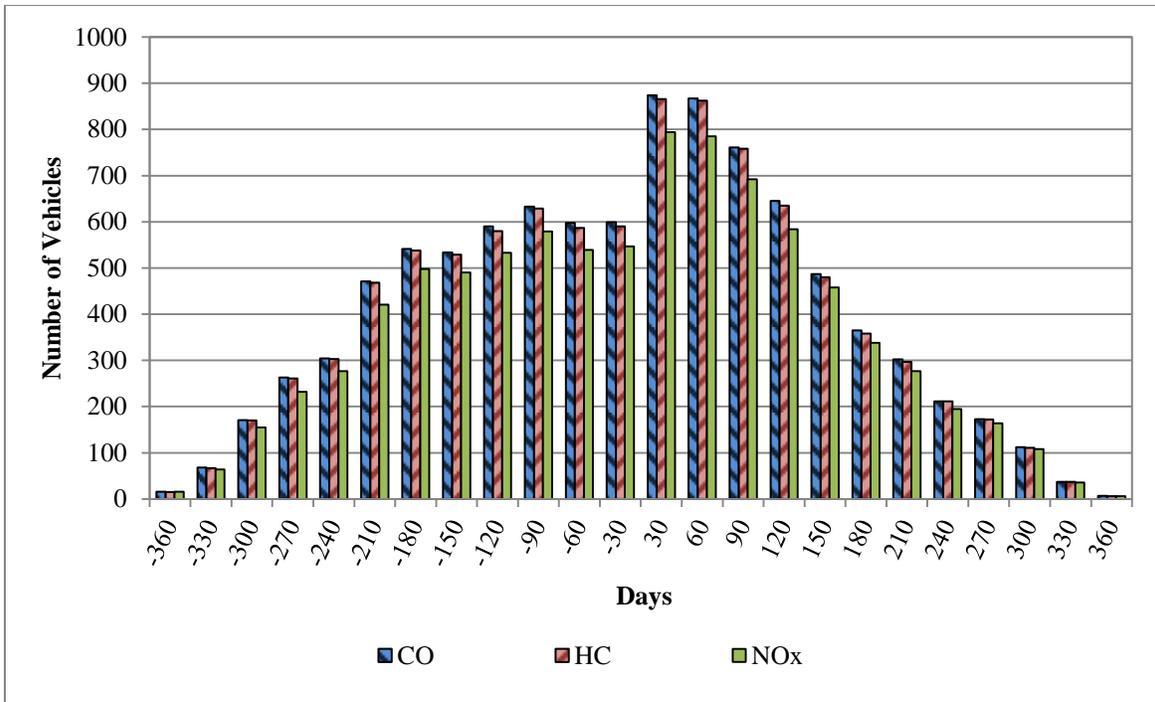
Figure 4-38 Histogram of number of vehicles per bin 'before' and 'after' repair for vehicles that failed the emission inspection test
