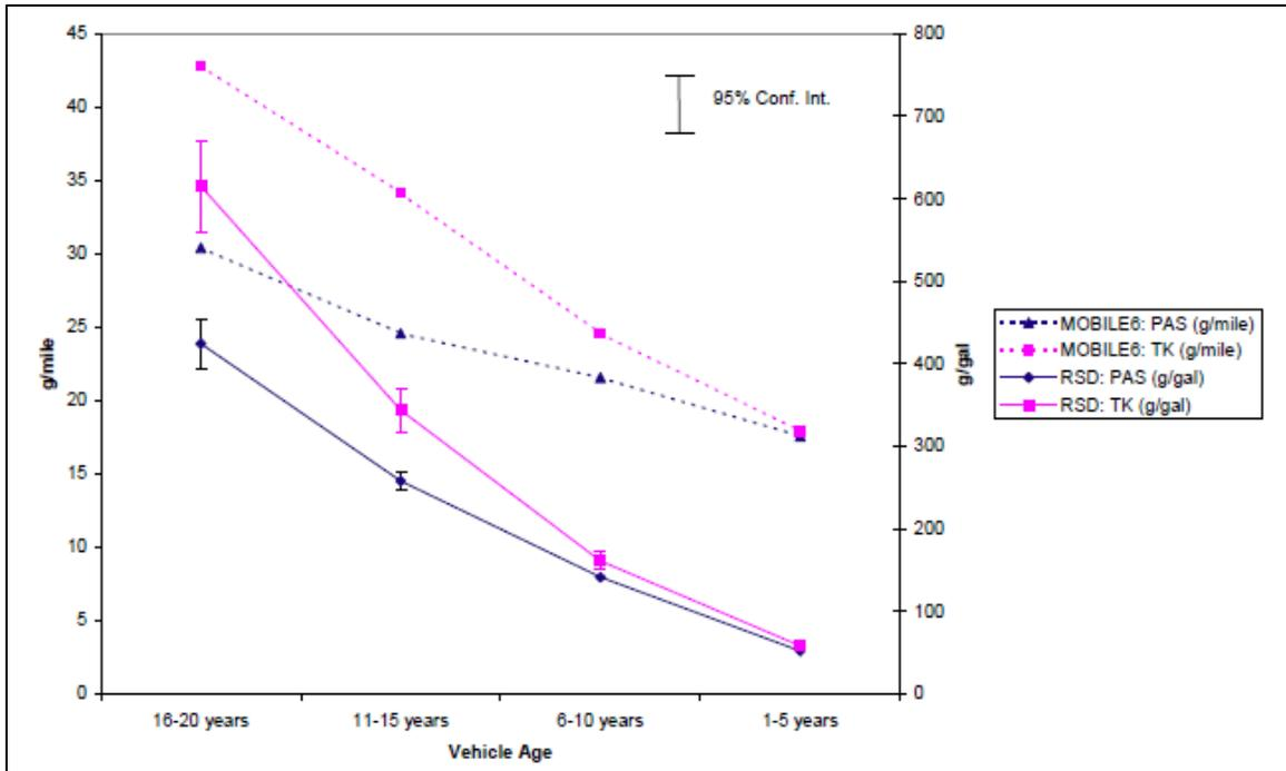
Figure 2-7 Mean CO emissions as a function of vehicle age of RSD data (g/gal) and from MOBILE6 (g/mile): Denver, 1999 – 2001
