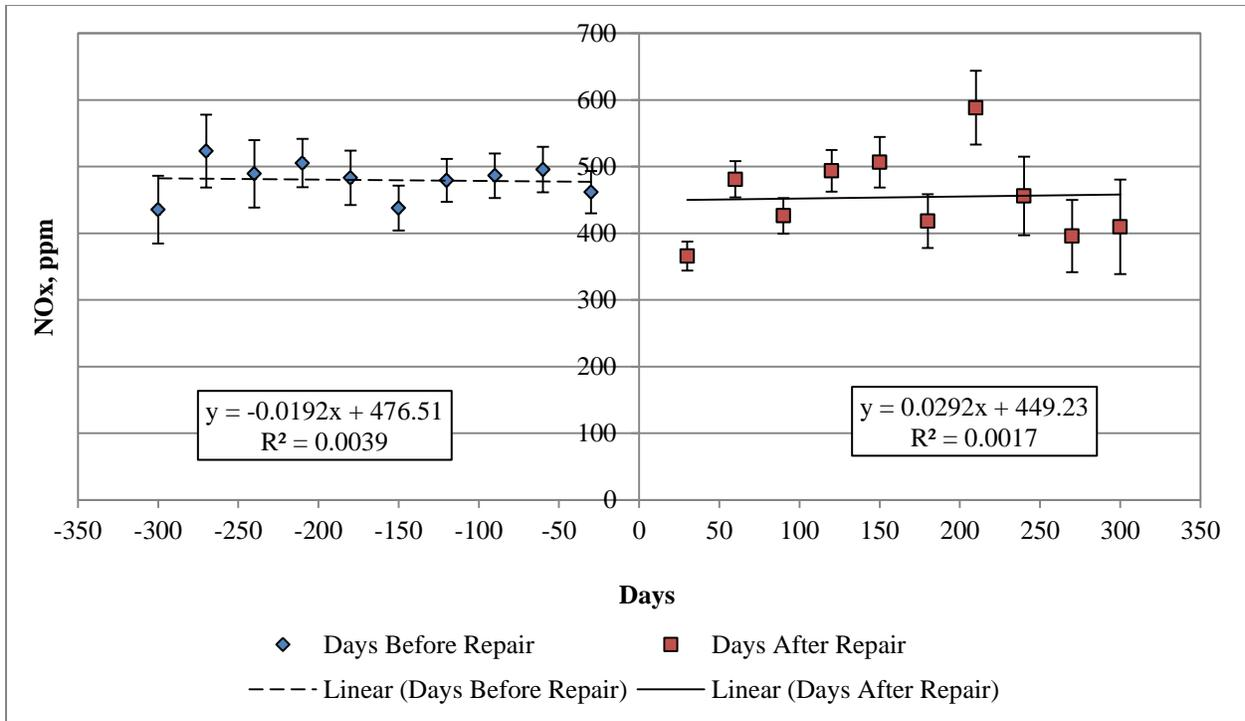
Figure 4-37 NOx measurements 'before' and 'after' repair for vehicles that failed the emission inspection test
