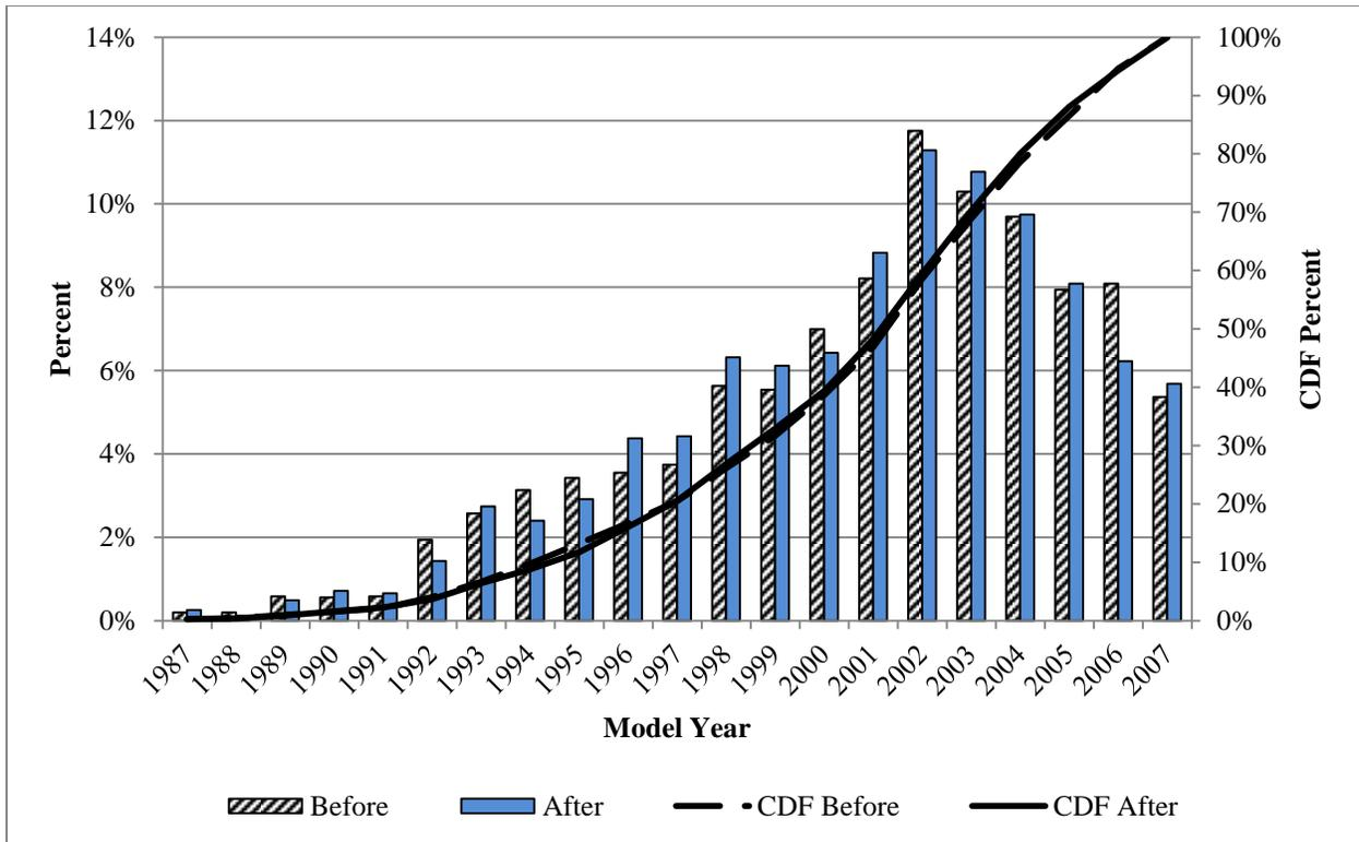
Figure 4-25 Model year distribution and CDF function of 'before-and-after' repair sample for vehicles that failed the emission inspection test
