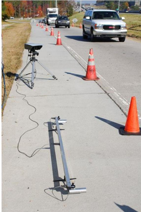
*Figure 3-5 Speed Acceleration Bar*
