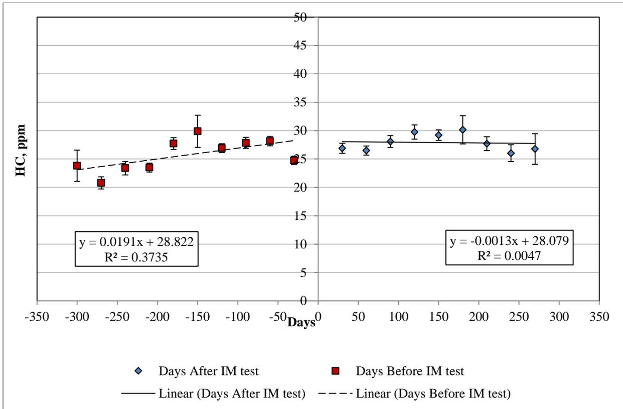
Figure 4-16 HC days before and after emission test for vehicles that did not fail the emission inspection test
