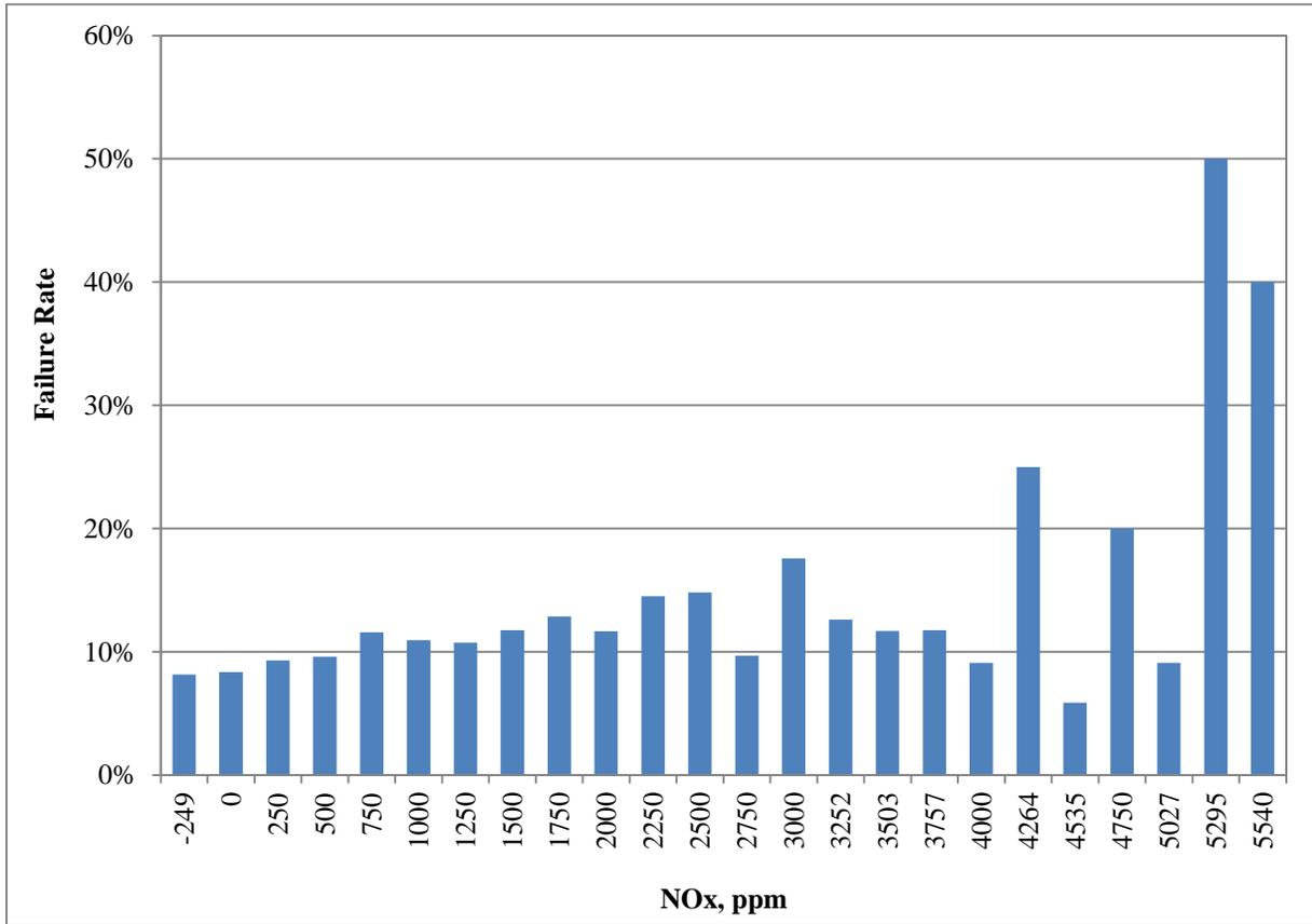
*Figure 5-9 Emission test failure rate vs vehicle emission remote sensing nitrogen oxides readings*
