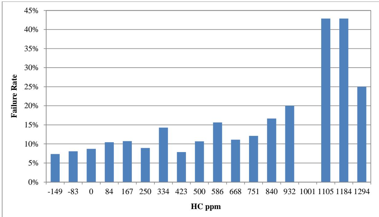
Figure 5-6 Emission test failure rate vs vehicle emission remote sensing hydrocarbon readings
