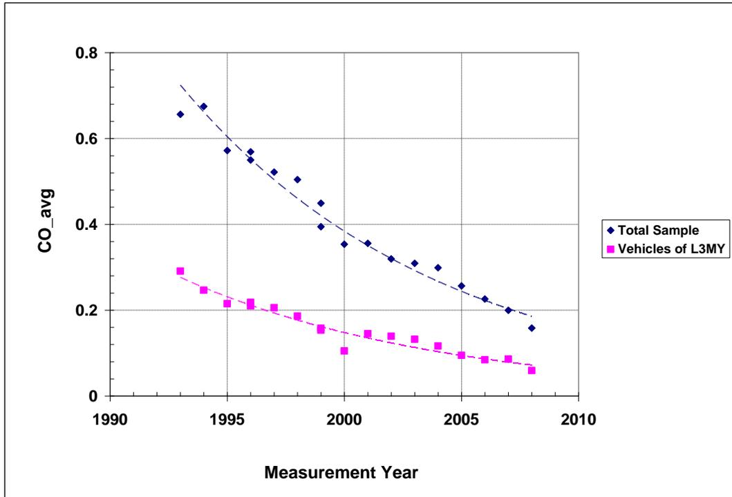
*Figure B-8 CO average of total sample and vehicles of latest three model years at various measurement years*
