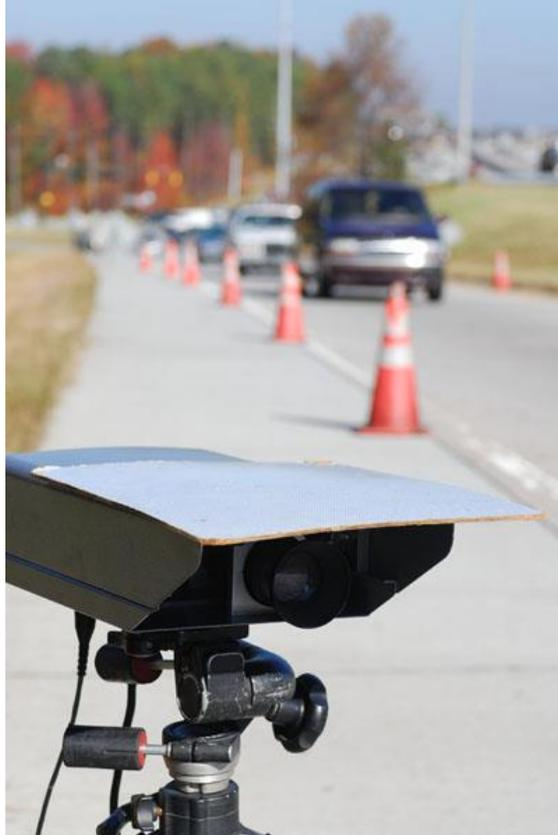
*Figure 3-14 Remote sensing camera*
