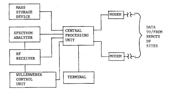
Figure 8-3. Recommended Local Control Configuration
