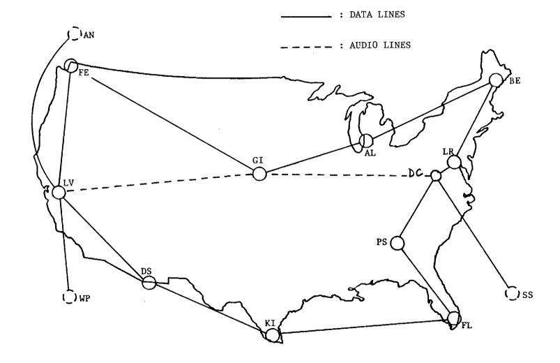
Figure 7-1. A Series-3000-Based Store-and-Forward Network.
