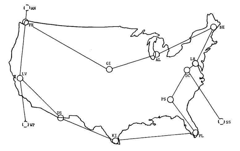
Figure 5-3. Alternative D: A Multi-Drop, Store-And-Forward Series 1000 Network.
