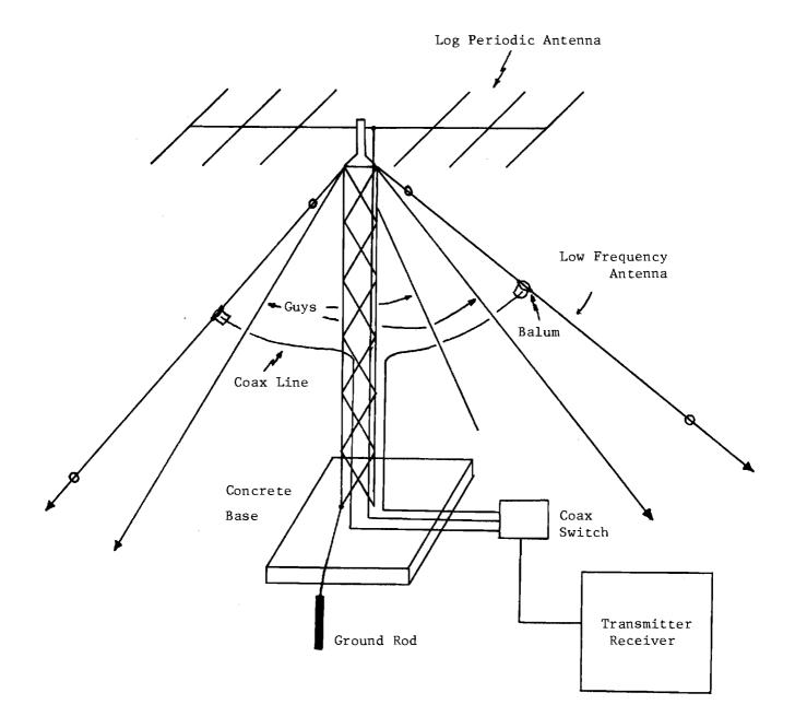
Figure 5-10 Antenna Configuration for HF Communication System
