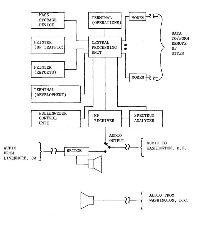
Figure 8-2. Recommended Secondary Control Site Configuration
