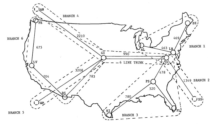
Figure 5-4. Alternative E: A Multi-point Network of Series 3000 Lines.
