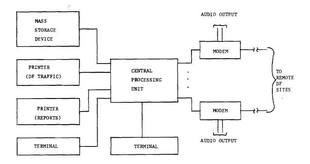
Figure 4-4 Network Control Configuration for Alternate Audio/Data Operation with Automatic Switching for Point-to-Point Configurations
