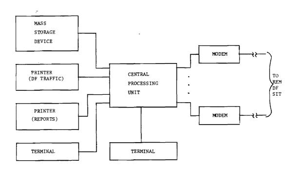
Figure 4-3 Network Control Configuration for Low Speed, Data Only Systems
