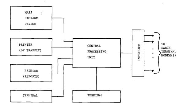
Figure 4-6 Network Control Configuration for Simultaneous Audio and Data
