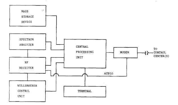
Figure 4-8 Local Control Configuration for Alternate Audio/Data Using Modem Switching
