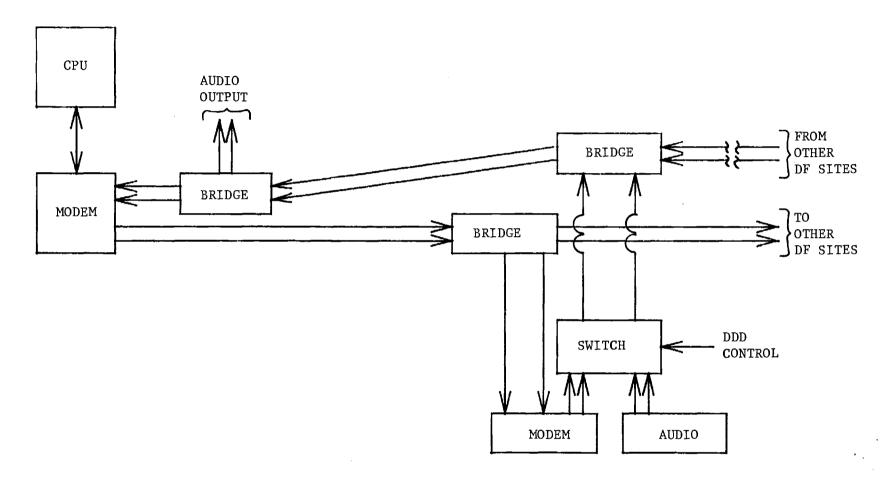
Figure 4-5 Audio/Data Selection by Remotely Controlled Switch
