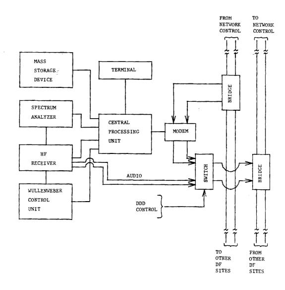
Figure 4-9 Local Control Configuration for Alternate Audio/Data Using Remotely Controlled Switching
