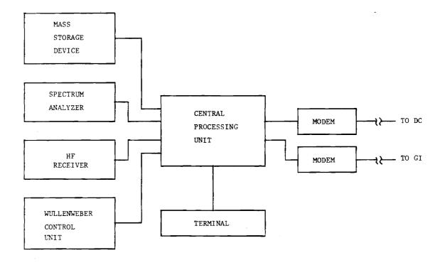
Figure 4-7 Local Control Configuration for a Low Speed, Data Only Network
