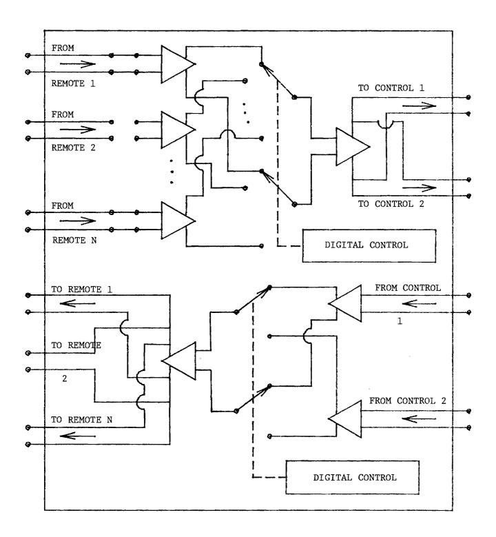
Figure 5-8. Schematic of A Digitally Controlled Analog Switch.
