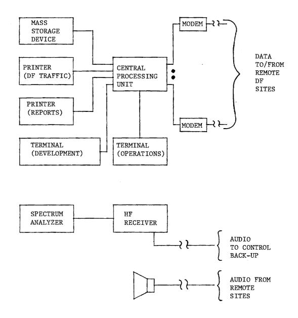
Figure 8-1. Recommended Primary Control Site Configuration
