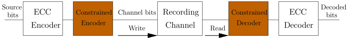
Figure 1: Block diagram of a digital recording system. Our focus is on the design of the shaded blocks, namely the constrained encoder and decoder.
