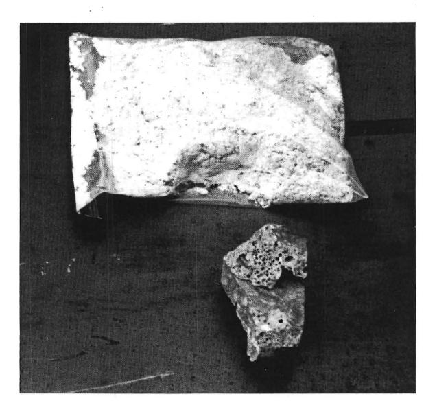
Figure 5. Samples (approximately 2 pounds each) of the pretest raw chrysotile asbestos and the post test vitrified solid residue
