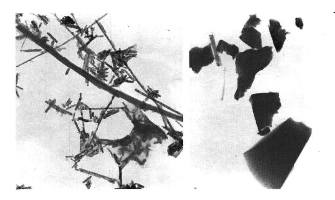
Figure 6. Transmission Electron Microscope (TEM) photographs of the pretest asbestos fibers and the post test vitrified solid residue.
