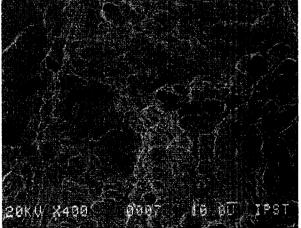
FIGURE 6(c). SEM micrograph showing brittle fracture FIGURE 6(d). SEM micrograph showing ductile fracture region of DSS sample with HT4 in WW3.
