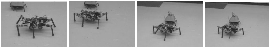
Figure 7.1: Photographs of the Wave Gait sequence of Byrobot
