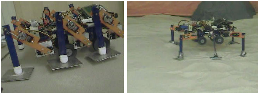
Figure 2.8: Mars Sand Shoes in place on Byrobot
