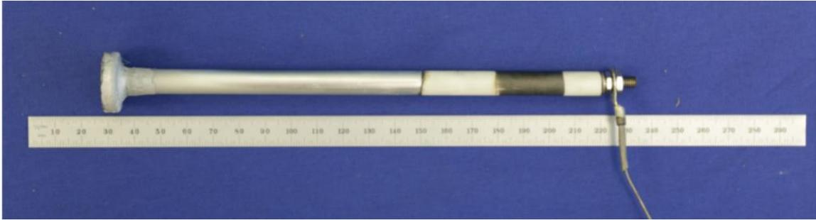
**Figure 19: Axial Plate Langmuir Probe**
