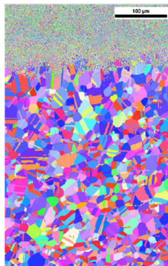
Fig. 2-5 Recrystallization occurring below the machined surface of AISI 304L stainless steel[27]
