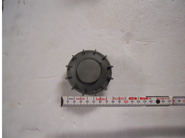
Figure 63: A photograph of a land mine used in the clutter experiments.
