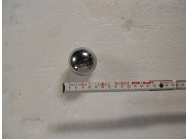
Figure 39: A photograph of a metal sphere used in the clutter experiments.
