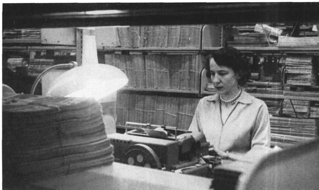
While another staff member cuts master catalogue cards on the Flexiwriter which in turn is used to make the seven to 12 cards needed for each new book in the library.
