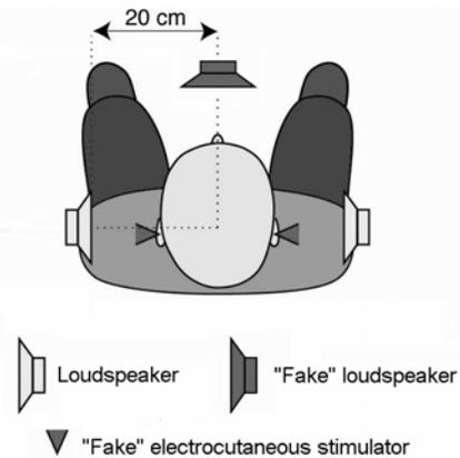
Figure 3. *Experimental setup. Auditory stimulation was delivered from left or right loudspeakers. Electrocutaneous stimulators and the front loudspeaker were not active during the experiment.*
