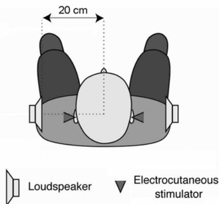
Figure 1. *Experimental setup. Auditory stimulation was delivered from either left or right loudspeakers, and electrocutaneous stimulation from either left or right earlobes.*
