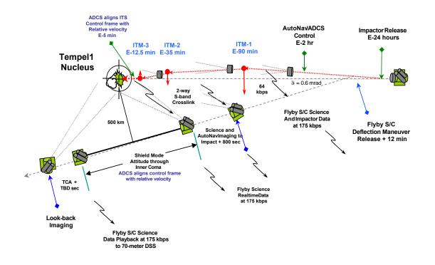
Figure 1. Schematic of Deep Impact Encounter with comet Tempel 1
