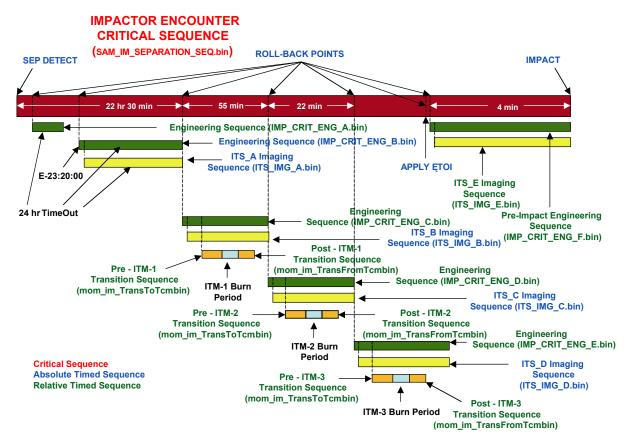
Figure 3. Impactor encounter sequence design schematic
