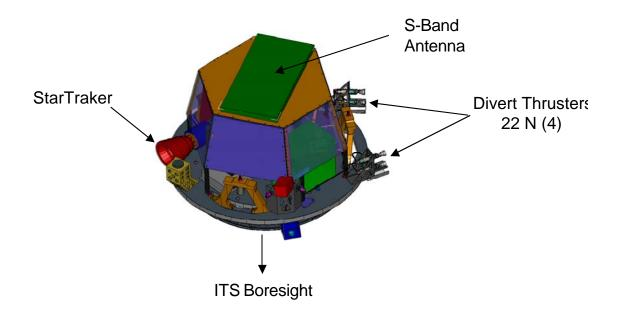
**Figure 2.** Impactor s/c flight system configuration<sup>1</sup>
