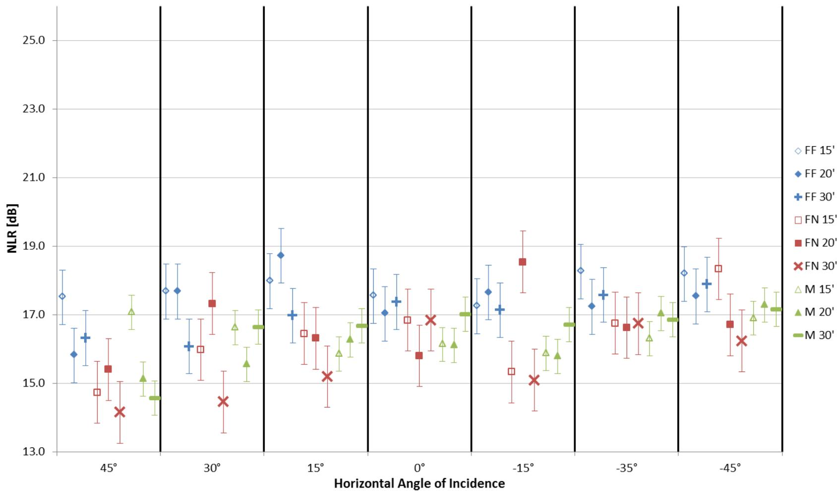
Figure 4.11: NLR values of the lift mounted speaker measurements
