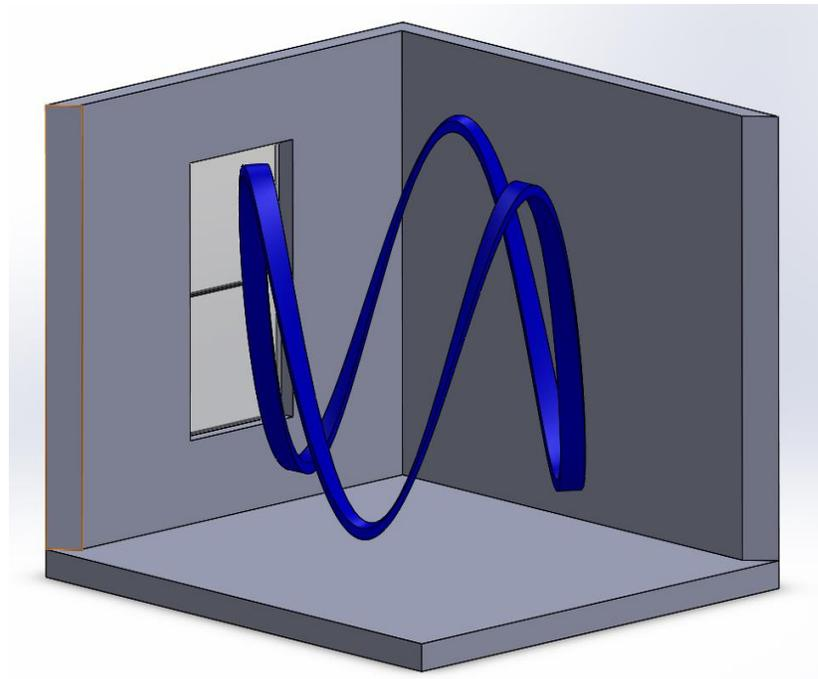
**Figure 3.15: Example idealized path of interior sound pressure level measurement using moving method**
