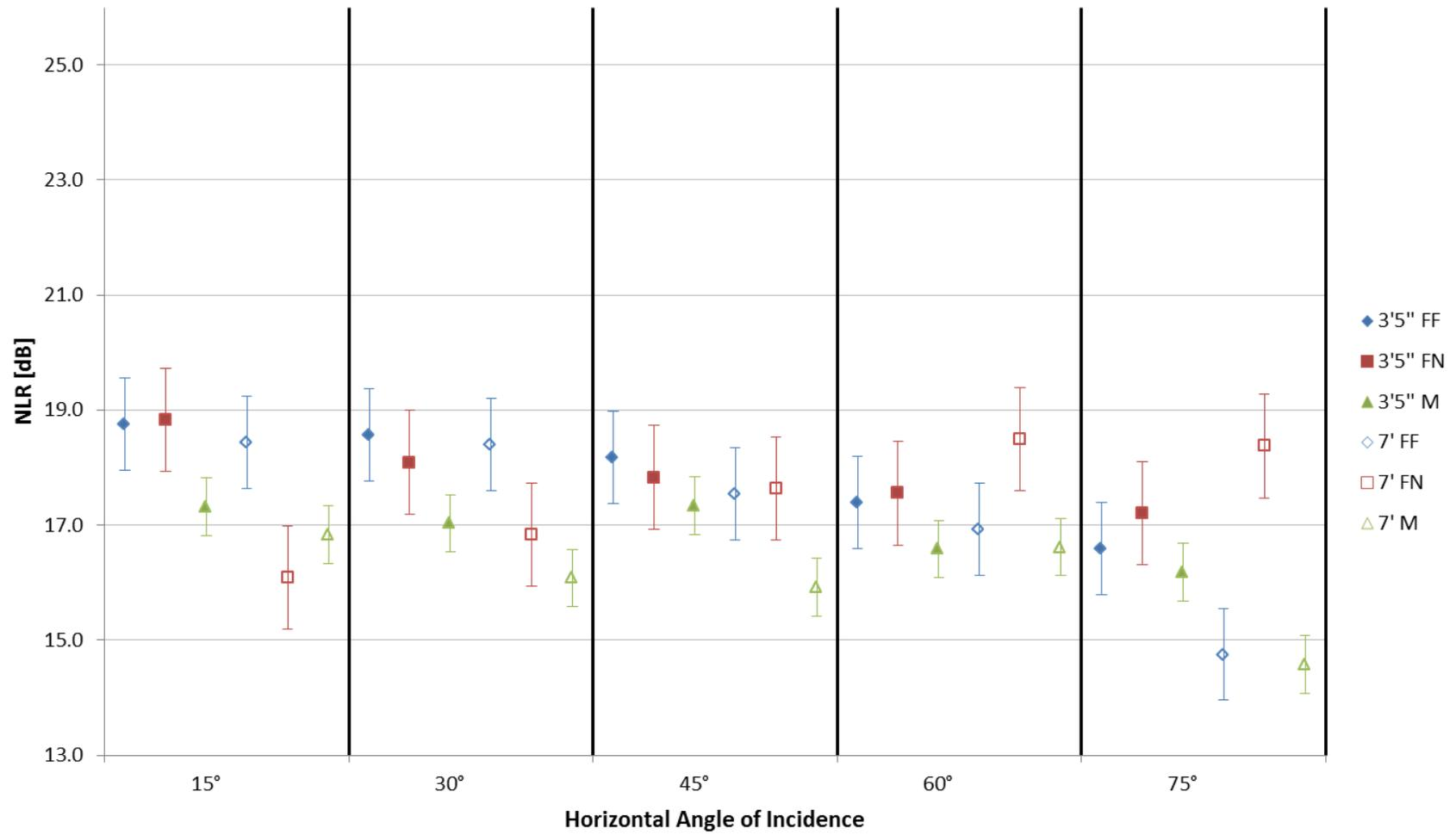
Figure 4.13: NLR values for radial locations of tripod mounted source with STC 25 window
