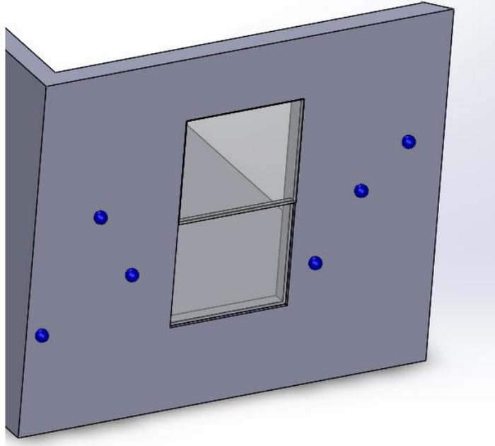
**Figure 3.11: Candidate microphone positions for the exterior measurements of the fixed flush method**
