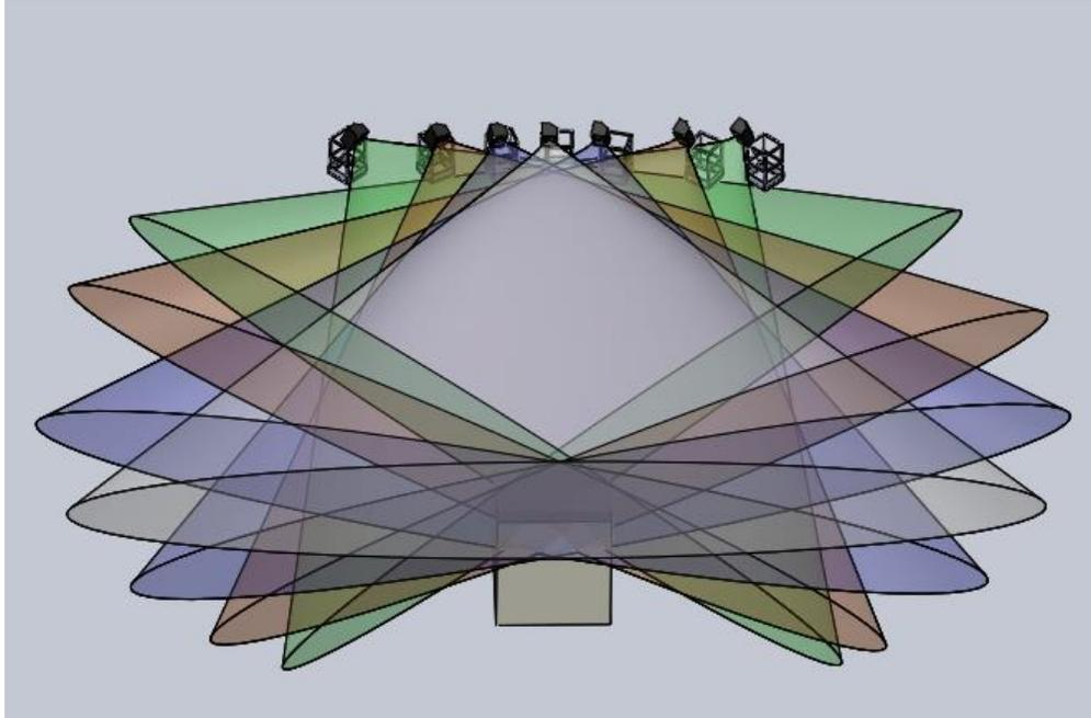
**Figure 4.5: Nominal radiation angles of the speaker elevated at 30' from an elevated rear view of the test house**
