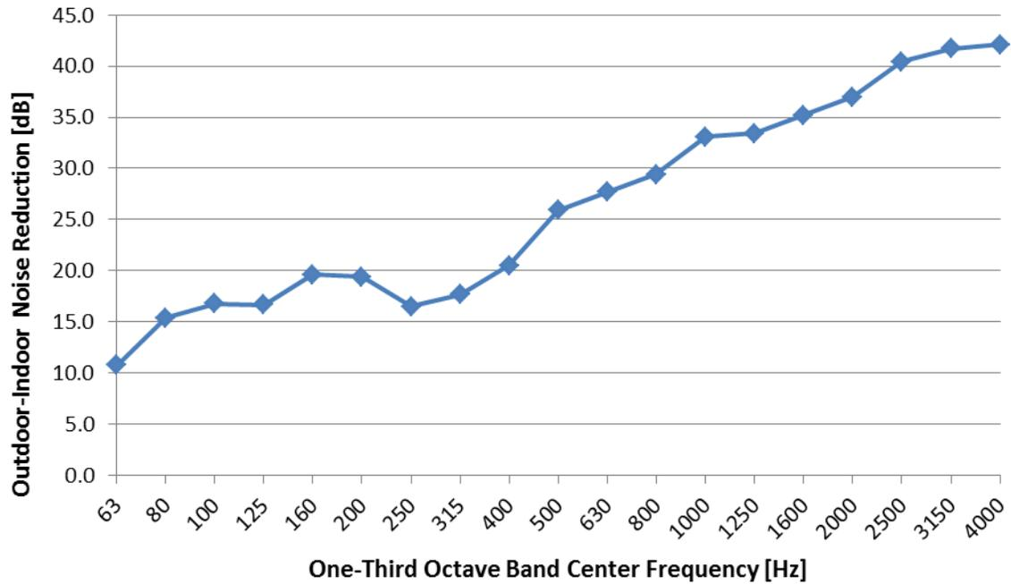
**Figure 2.1: NR for an example measurement**
