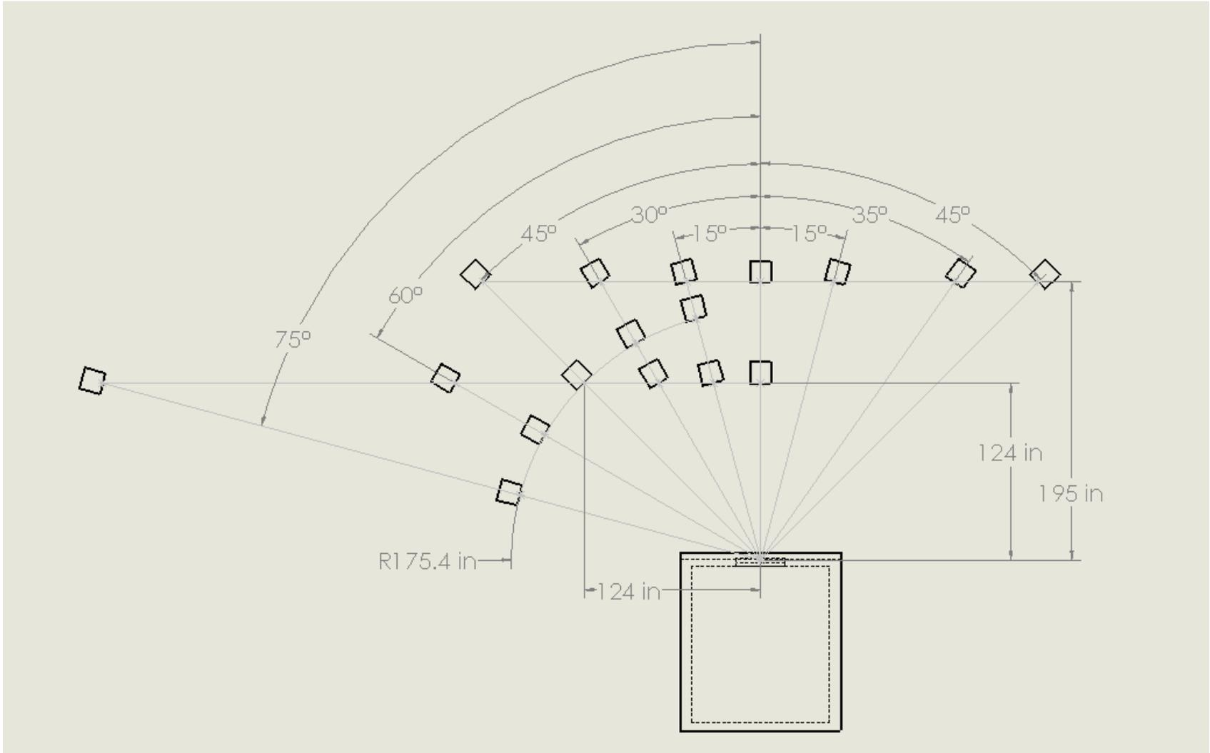
Figure A.5: Drawing of sound source locations
