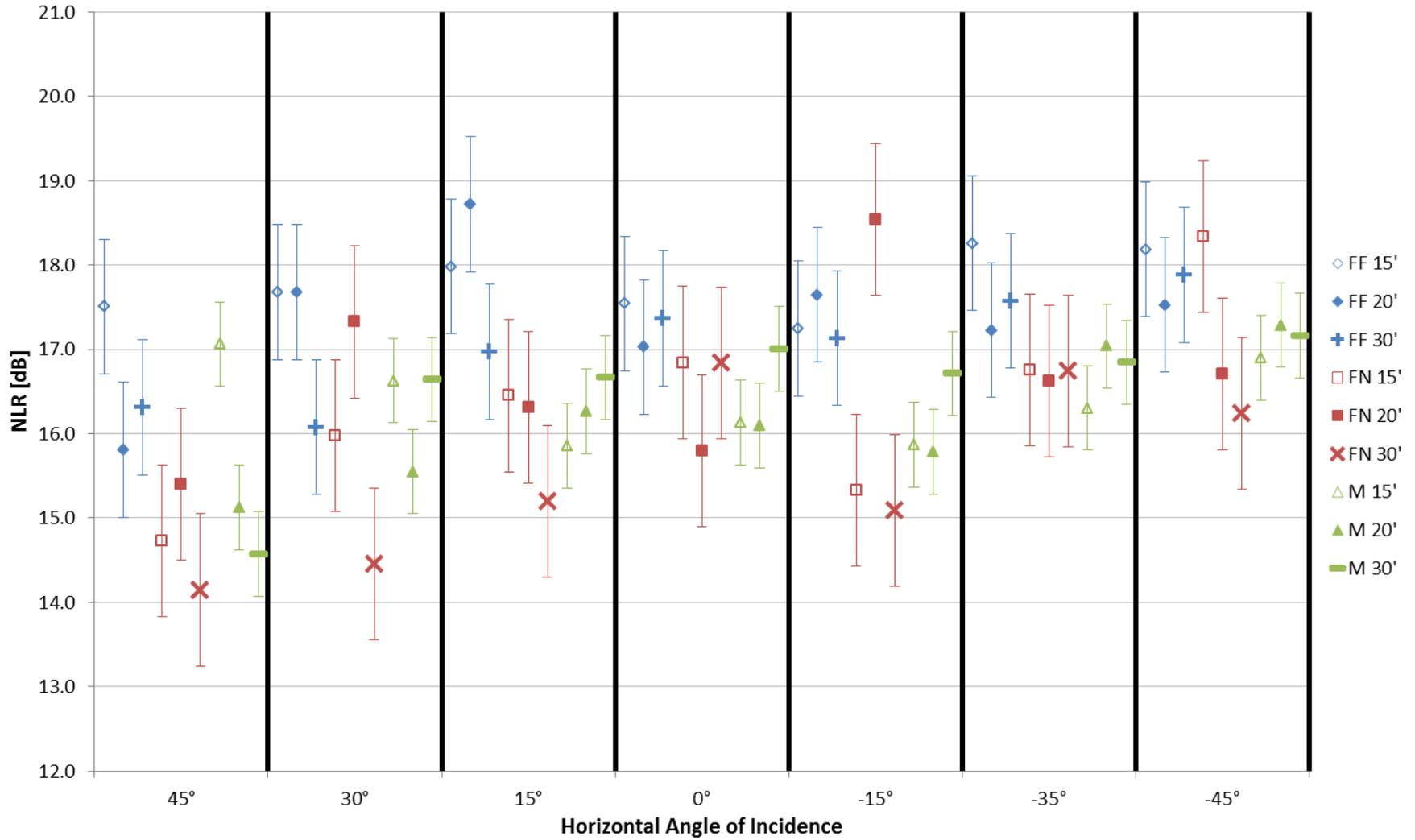
Figure 4.4: NLR values of the lift mounted speaker measurements
