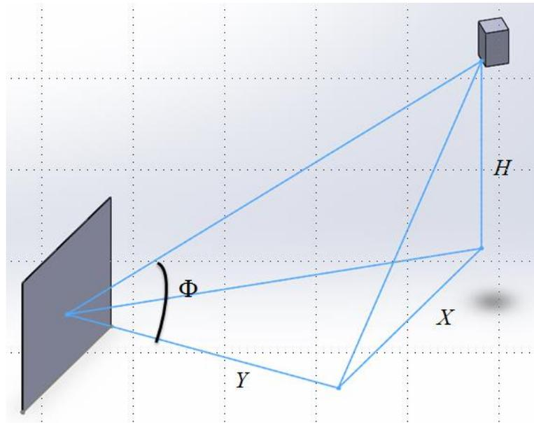
**Figure 4.10: Diagram of three-dimensional angle of incidence,  $\Phi$**
