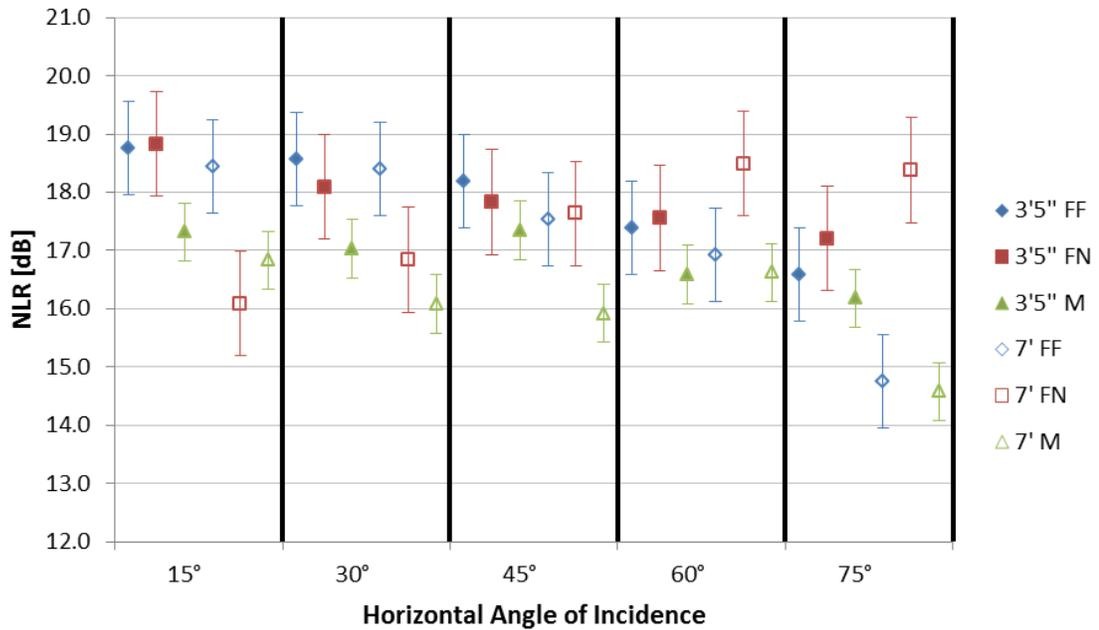
Figure 4.2: NLR values for radial locations of tripod mounted source with STC 25 window
