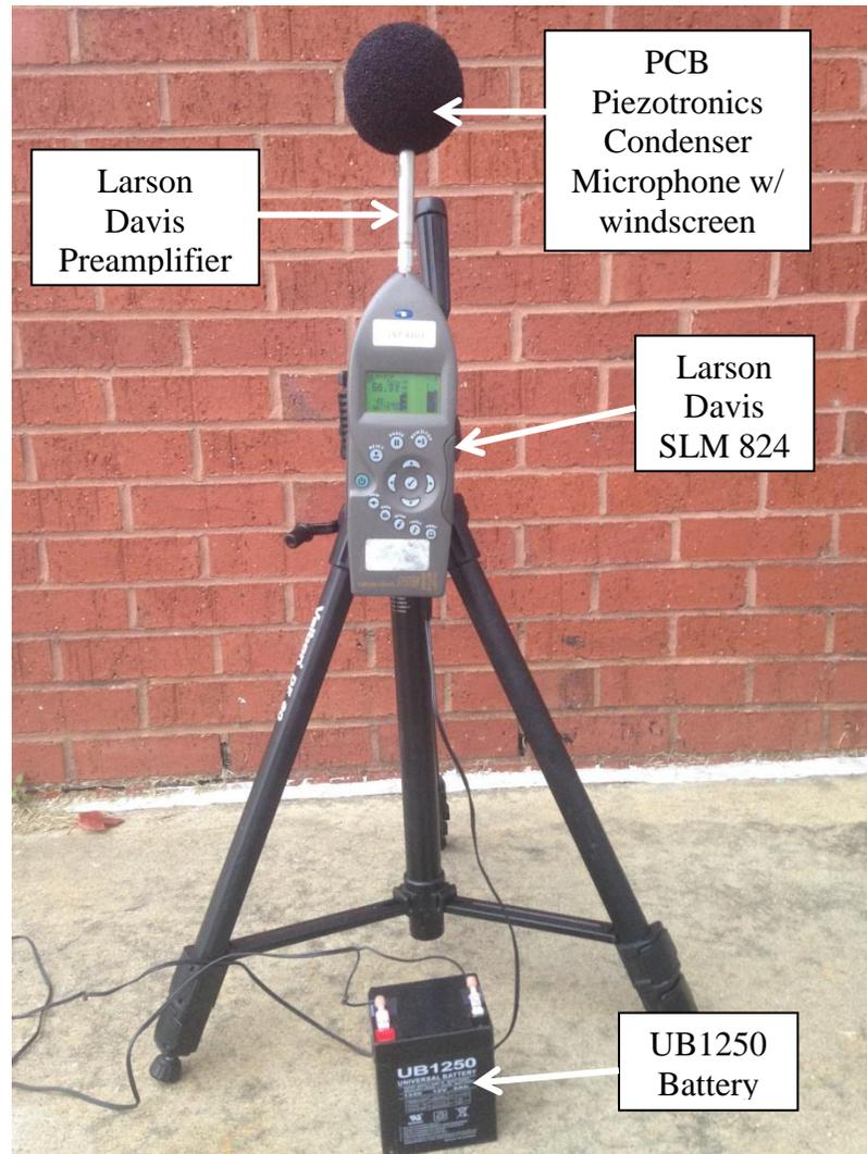
**Figure 3.6: Picture of measurement devices used in testing**
