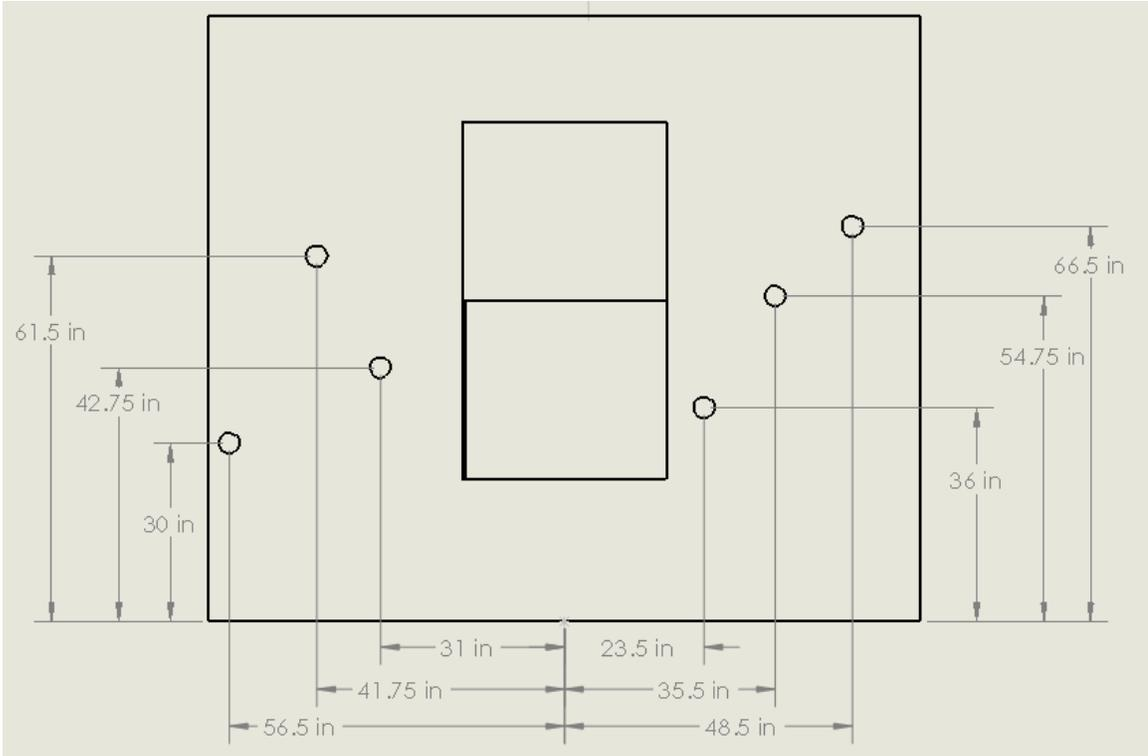
**Figure A.3: Drawing of exterior fixed flush measurement locations**
