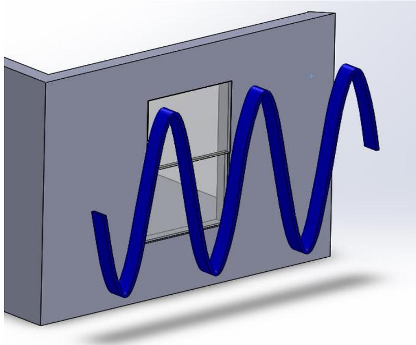
**Figure 3.14: Example idealized path of exterior sound pressure level measurement using moving method**
