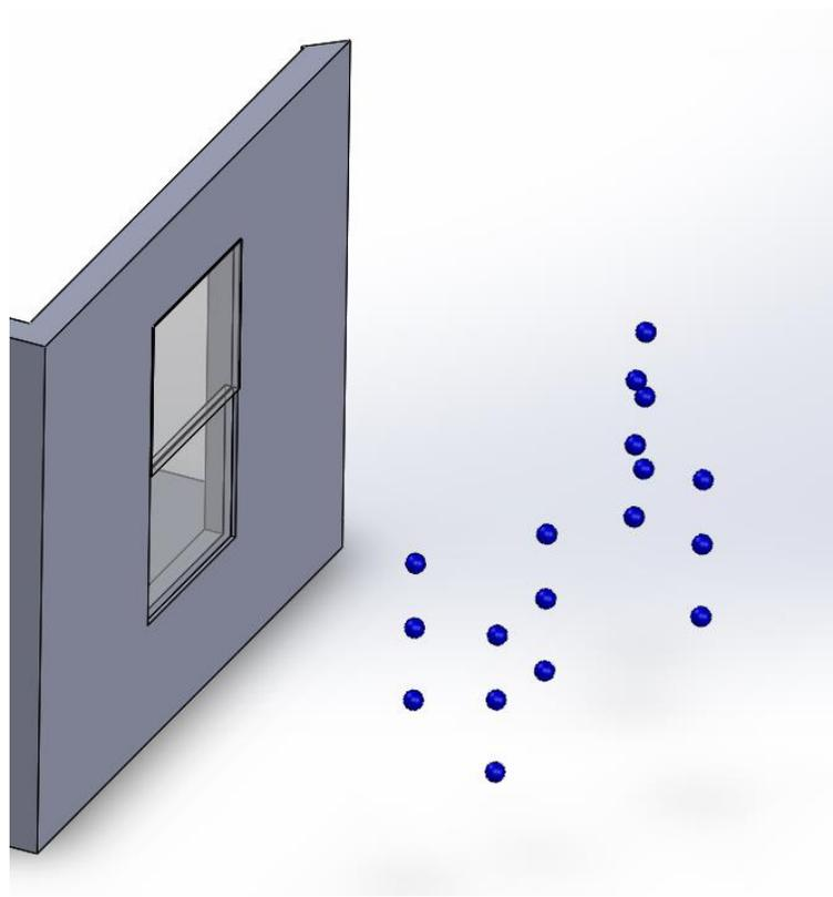
**Figure 3.8: Candidate microphone positions for the exterior measurements of the fixed near method**
