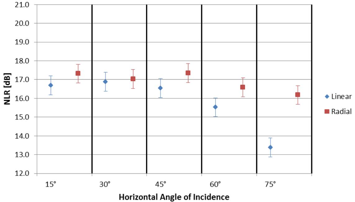
**Figure 4.3: NLR values for the linear and radial locations for 3'5" source with STC 25 window and moving method**
