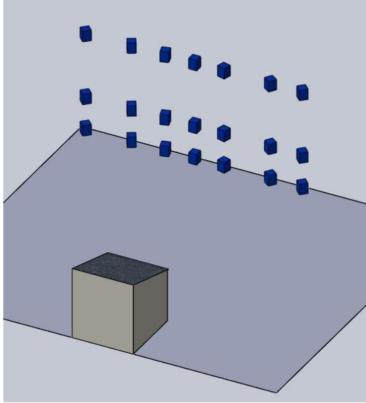
**Figure 3.17: Lift mounted speaker locations from a rear view of the test house**
