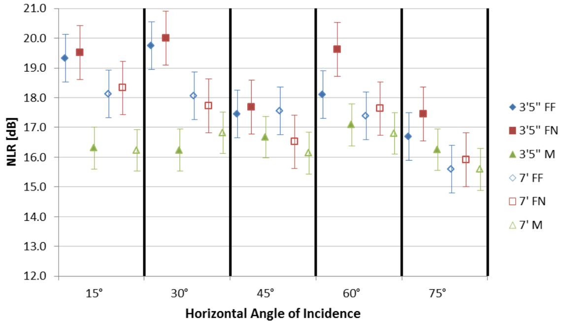
**Figure 4.8: NLR values for radial locations of tripod mounted source with STC 31 window**
