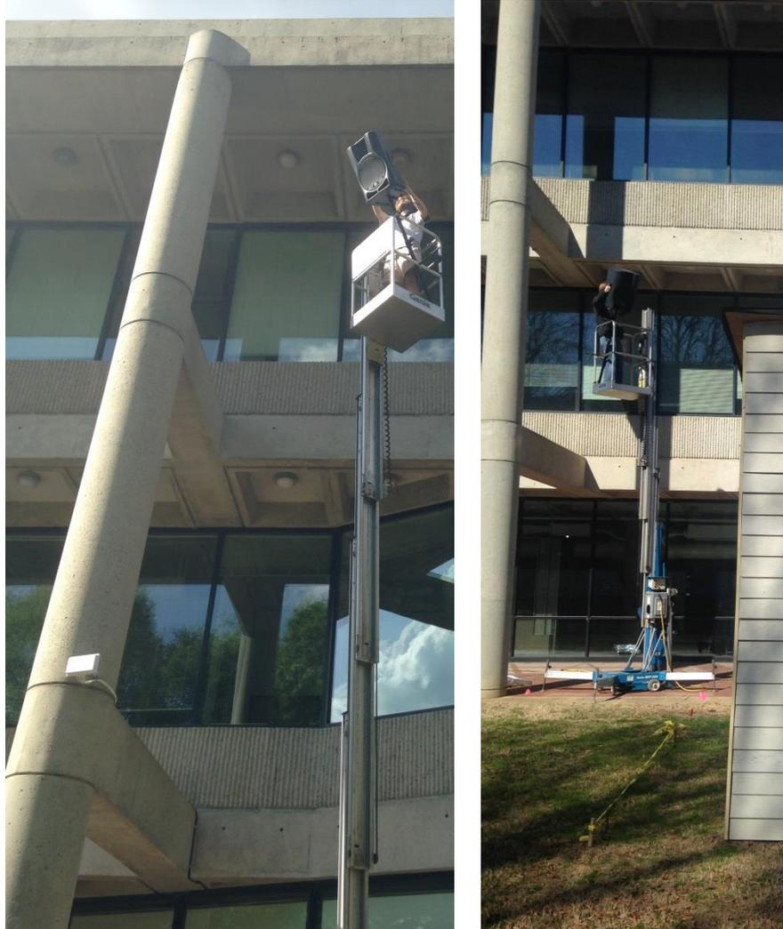
**Figure 3.21: (a) picture with speaker at source height of 30' and (b) picture with speaker at source height of 15'**
