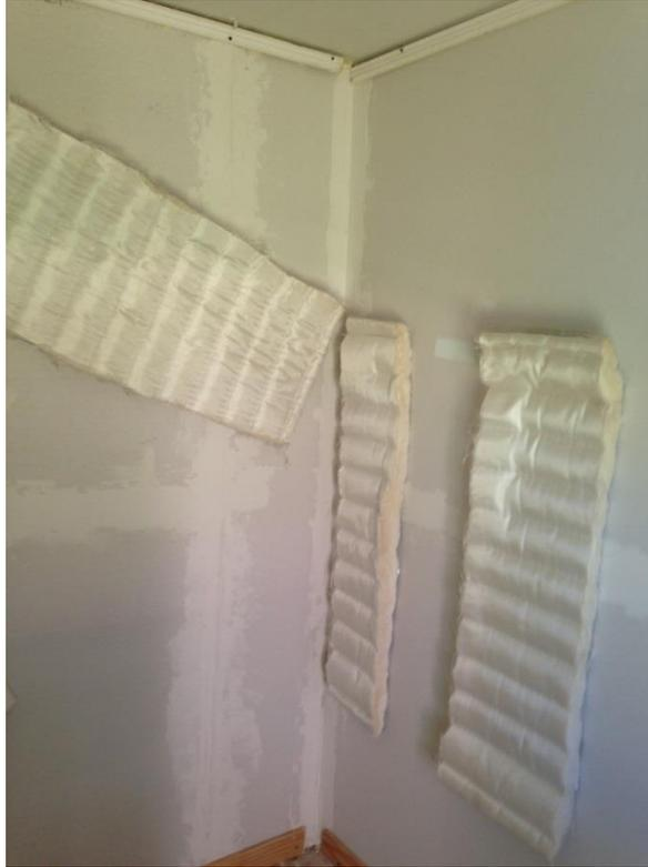
**Figure 3.4: Example of random placement of Insul-Quilt mounted on a wall of the test house**
