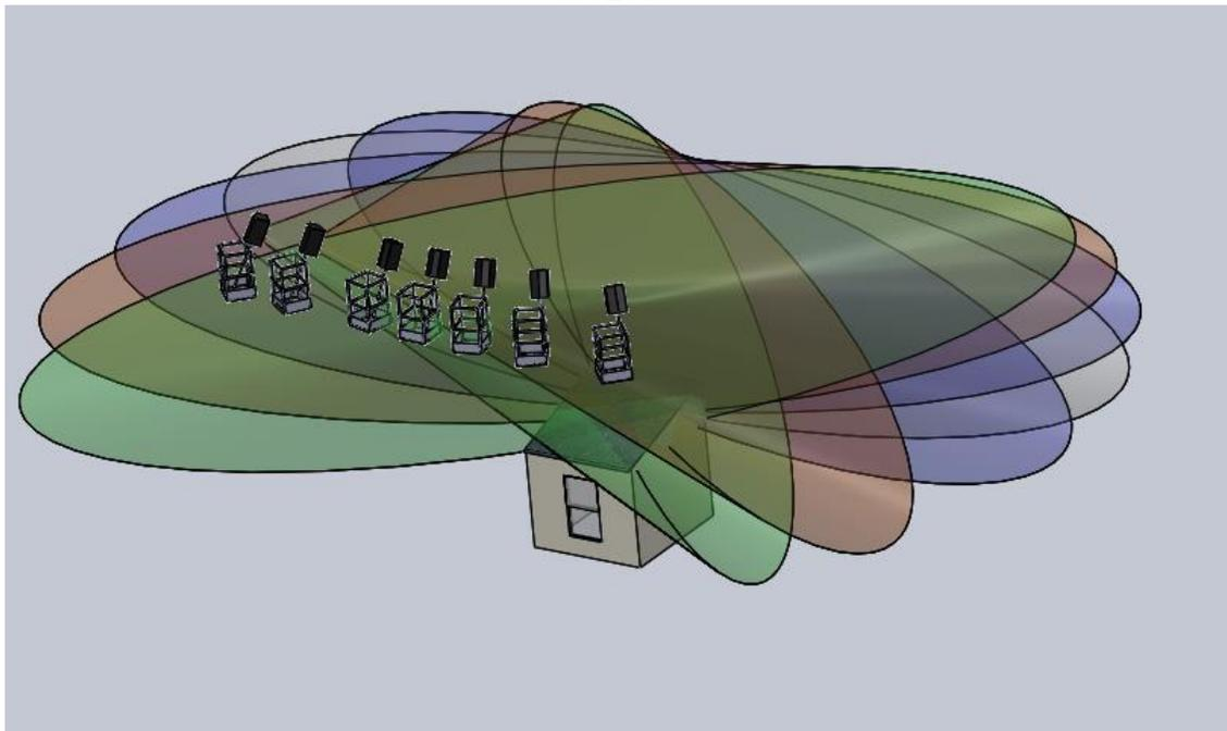
**Figure 4.6: Nominal radiation angles of the speaker elevated at 30' from a front corner view**
