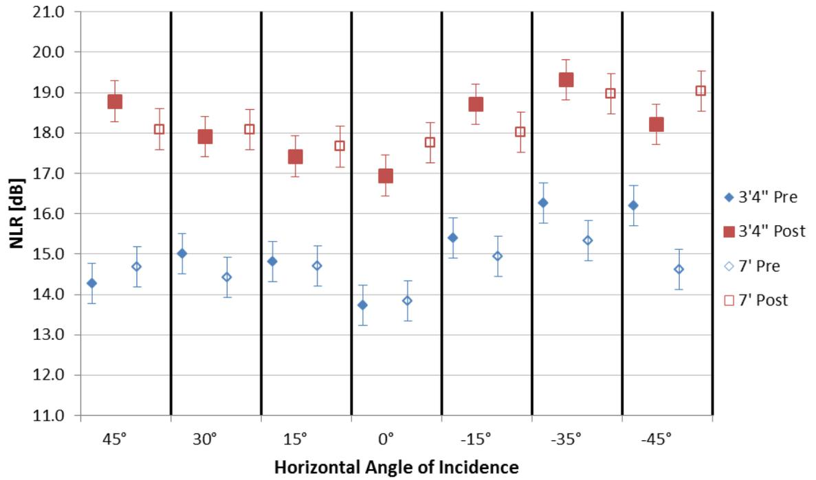
Figure 4.17: NLR values measured before and after foam application
