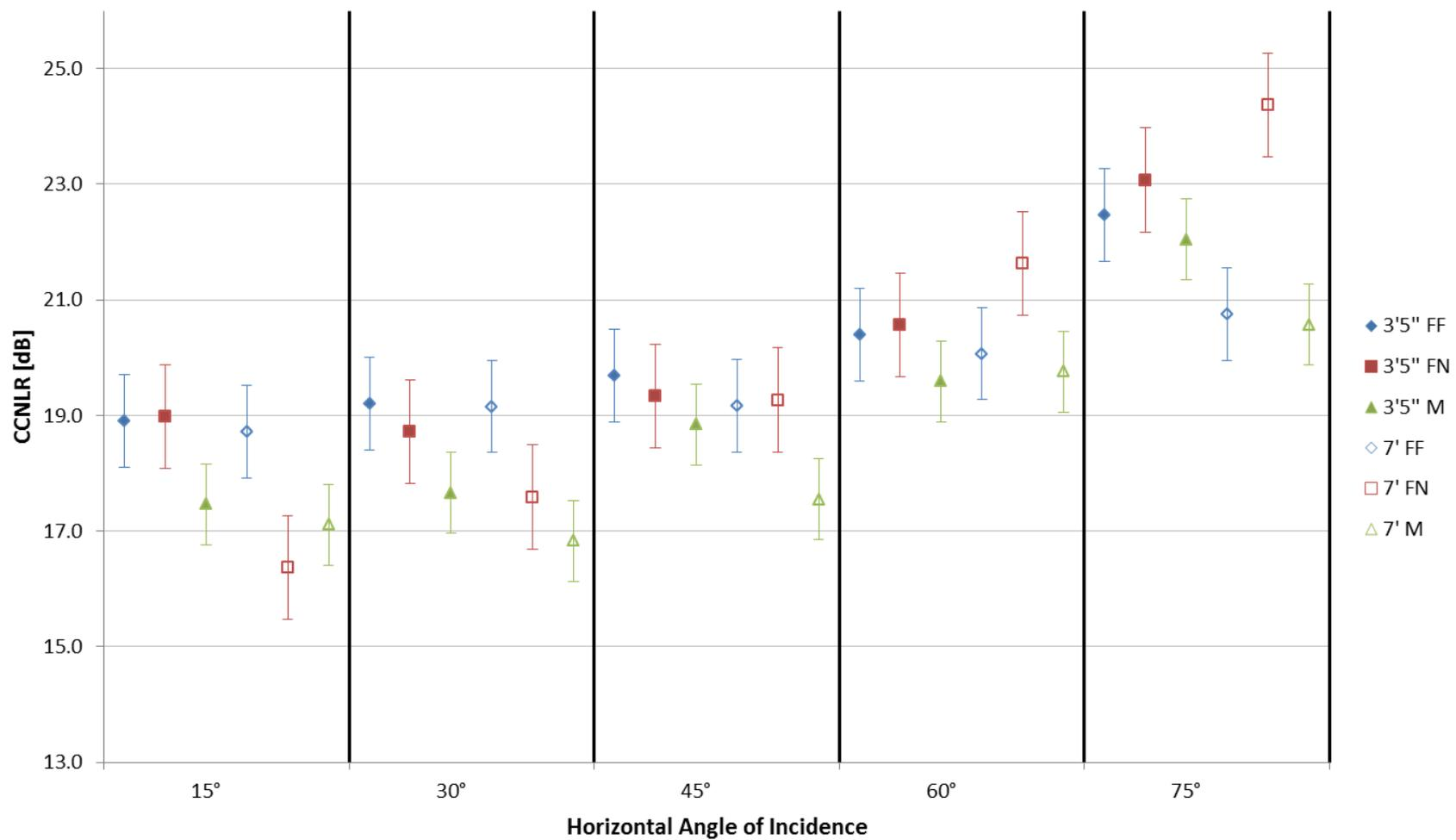
Figure 4.14: CCNLR values for radial locations of tripod mounted source with STC 25 window
