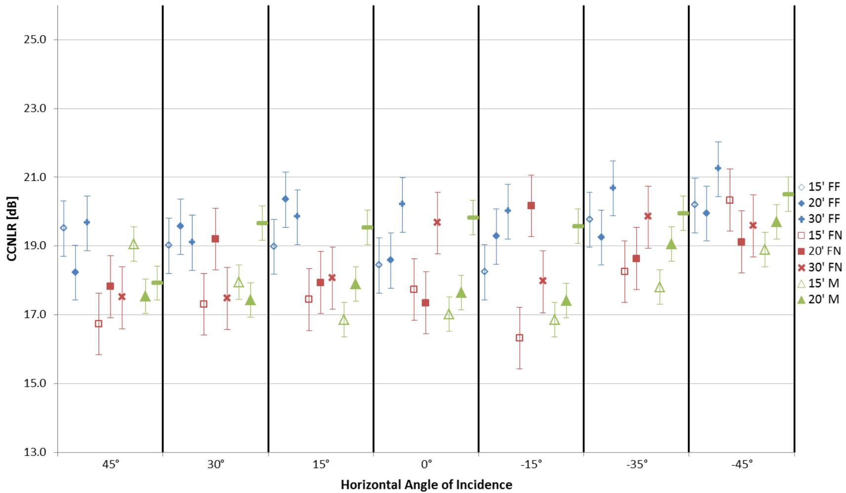
Figure 4.12: CCNLR values of the lift mounted speaker measurements
