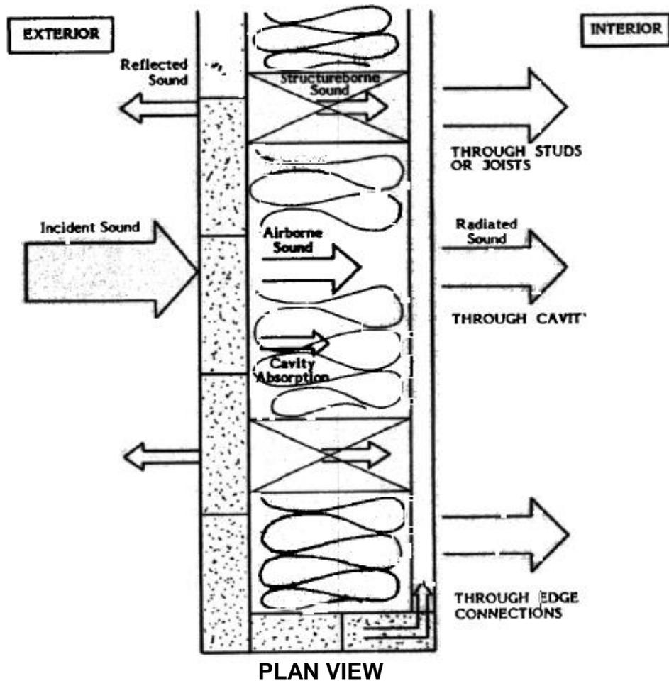
Figure 1.1: Demonstration of possible sound paths inside a building reproduced from [4]
