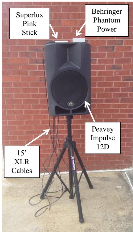
**Figure 3.5: Picture of sound source equipment used in testing**
