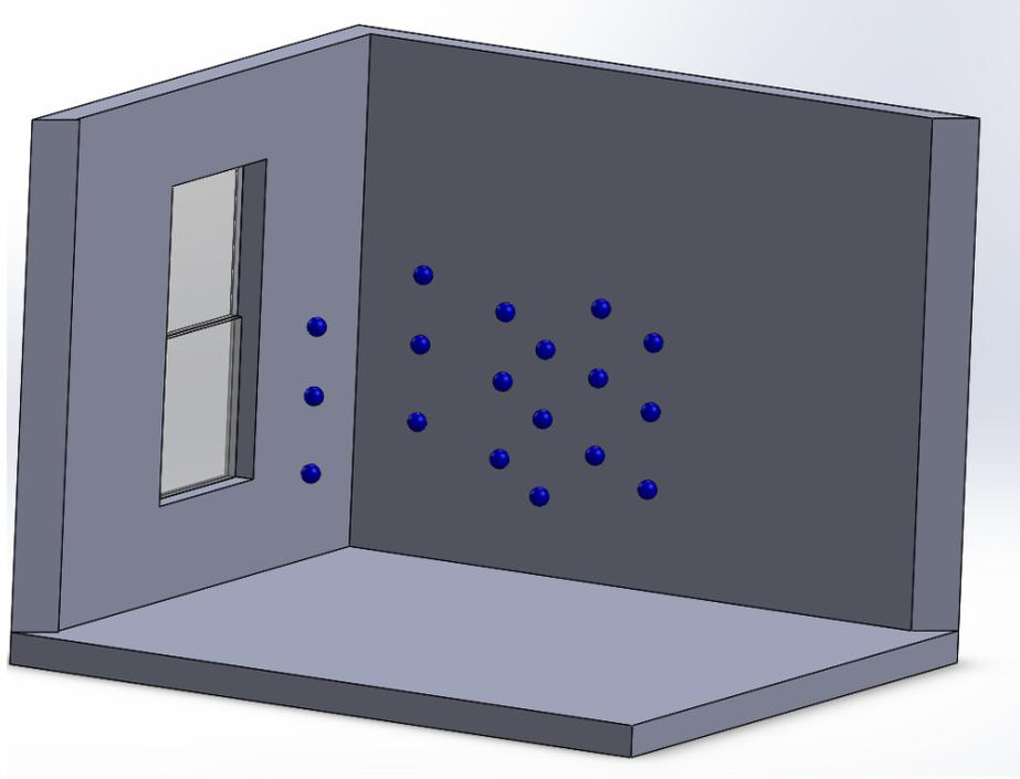
**Figure 3.9: Candidate microphone positions of the fixed interior measurements**
