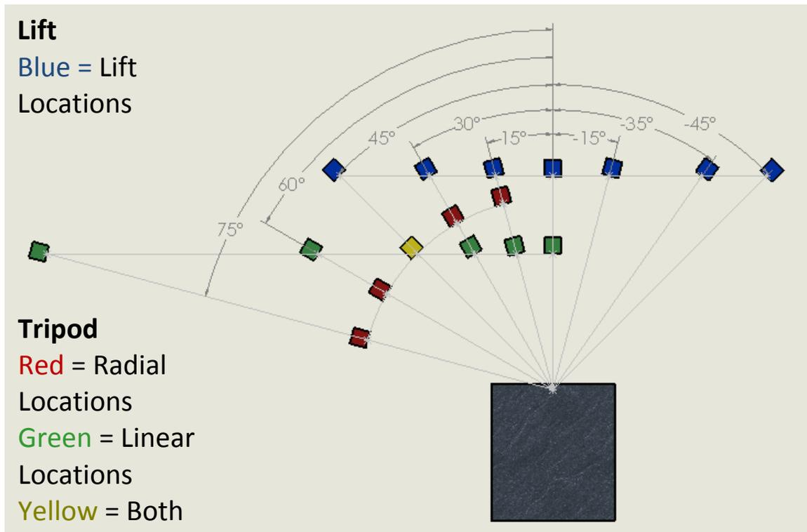
Figure 3.19: Tripod mounted speaker locations from a top view of the test house
