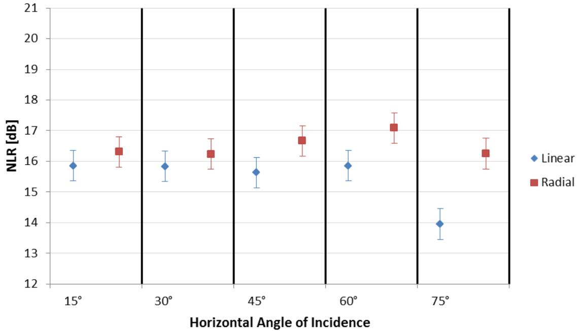
**Figure 4.9: NLR values for the linear and radial locations for 3'5" source with STC 31 window and moving method**
