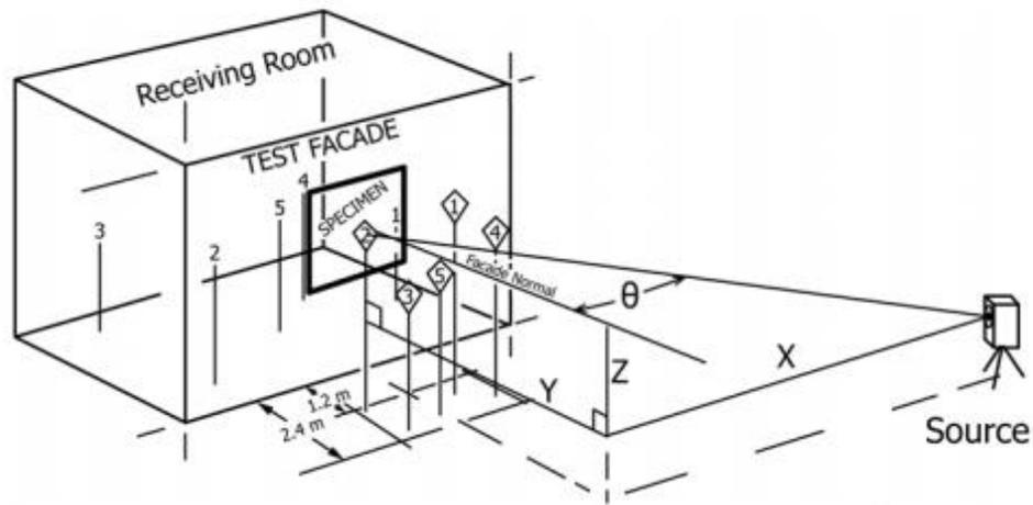
Figure 3.7: Geometry example of fixed near method reproduced from [21]
