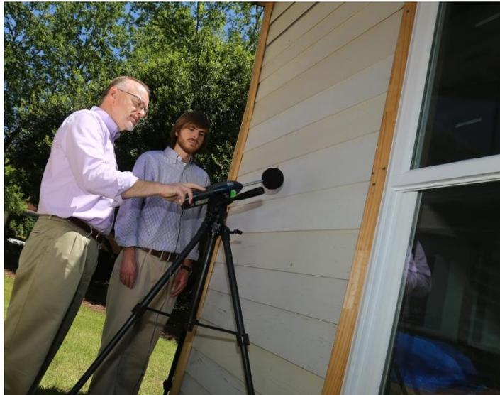
**Figure 3.12: Example of fixed flush exterior sound pressure level measurement location**
