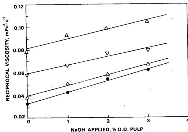
Fig. 3 The reciprocal of pulp viscosity is linearly related to caustic charge in the oxygen stage, regardless of pulping conditions. Symbols are as shown in Table 3.
