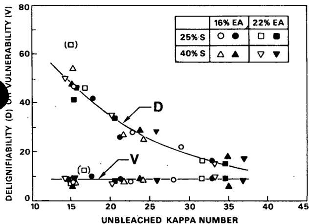
Fig. 2 The delignifiability (D) of a pulp in an oxygen stage depends on its unbleached kappa number but not on the conditions used to prepare it. Its vulnerability to depolymerization (V) depends on neither.
