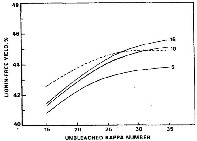
Fig. 8 At 25% sulfidity, 16% EA and with no AQ, terminating the cook at kappa number 35 gives the highest yield for all values of post-oxygen-stage kappa number, which is the parameter on the graph. Raising the sulfidity to 40% and adding 0.1% AQ (dashed line) decreases the optimum unbleached kappa number.
