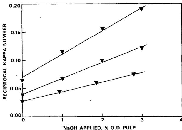
**Fig. 1** The reciprocal of the kappa number is linearly related to caustic charge in the oxygen stage, regardless of pulping conditions. Data shown are for cooks with 0.1% AQ and 22% EA at 40% sulfidity.
