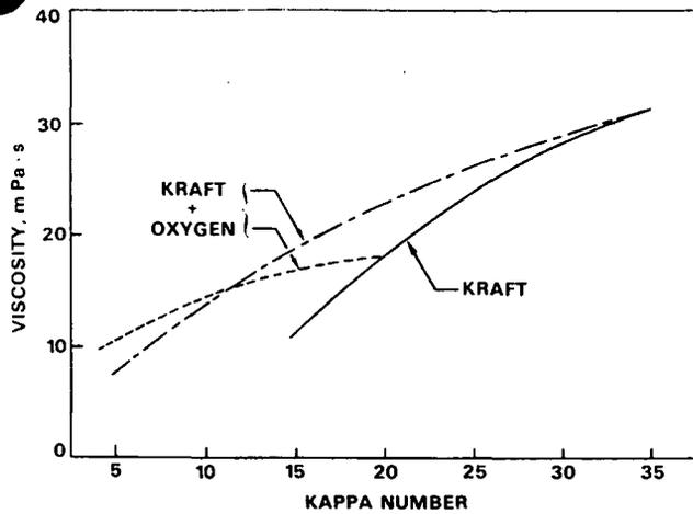
Fig. 5 For a kappa number of 12 or less after the oxygen stage, terminating the kraft cook at kappa number 35 gives lower viscosity than extending the cook to kappa number 20.
