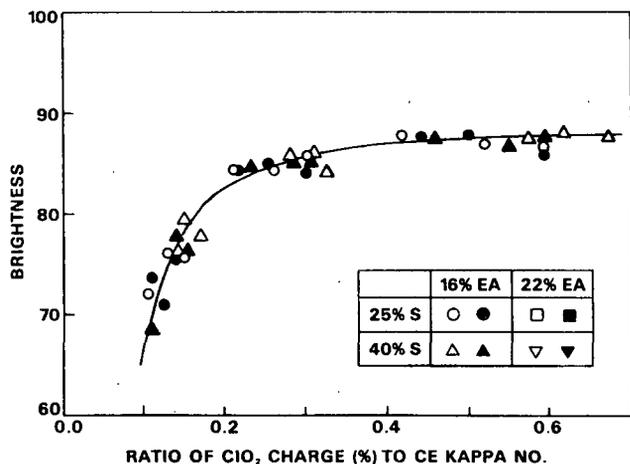
Fig. 4 Fully bleached brightness depends on the ratio of the ClO<sub>2</sub> charge to the kappa number after caustic extraction but not on digester conditions.
