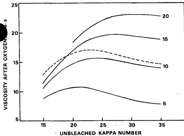
Fig. 6 At 25% sulfidity and 16% EA, the optimum unbleached kappa number depends on the post-oxygen-stage kappa number target, which is the parameter in the graph. Raising the sulfidity to 90% (dashed line) decreases the optimum unbleached kappa number.
