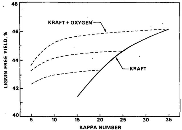
Fig. 7 Terminating the kraft cook at kappa number 35 gives higher yield after the oxygen stage than extending it to lower kappa numbers.
