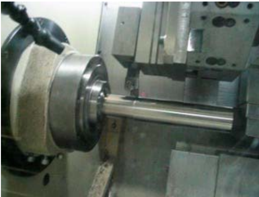
Figure 7-5. Experimental set up for the stability limit measurements in outward turning
