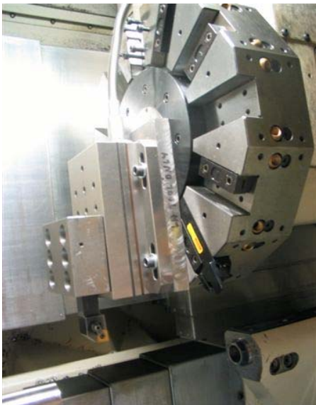
Figure 7-4. Dynamometer setup mounted on the tool post
