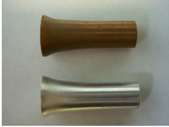
Figure 21: Final deformation states for recovered copper and aluminum samples from the Taylor rod-on-anvil impact tests.
