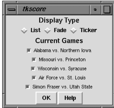
Figure 1: The main tkscore screen used to select display type and games. The display types are presented in random order upon startup to help avoid selection bias. If the fade or ticker display is selected, a speed selection bar appears. Initially all games are selected - a user can toggle the selection by clicking on the box next to the game.
