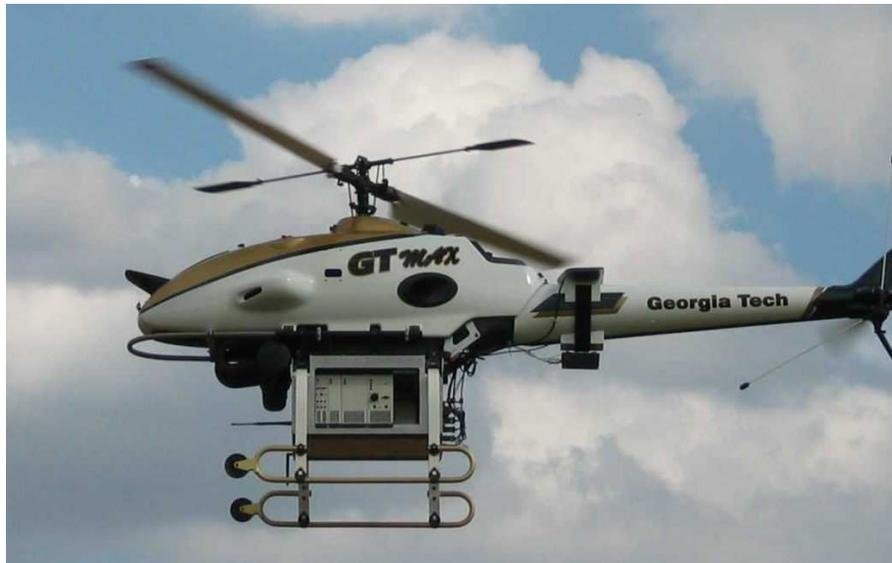
**Figure 54:** Georgia Tech unmanned aerial vehicle testbed- GTMax
