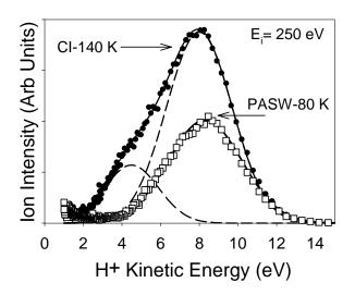
Figure 3.3 Proton kinetic energy distributions from CI and PASW
