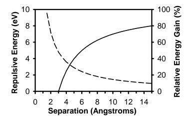
Figure 3.10 Coulomb repulsion between two point charges
