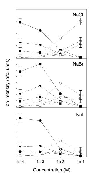
Figure 6.2 Concentration dependence of cluster yield from NaCl, NaBr and NaI
