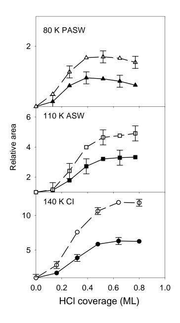
Figure 4.2 Cation yield as a function of HCl coverage
