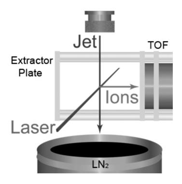
Figure 5.1 Schematic of liquid jet chamber
