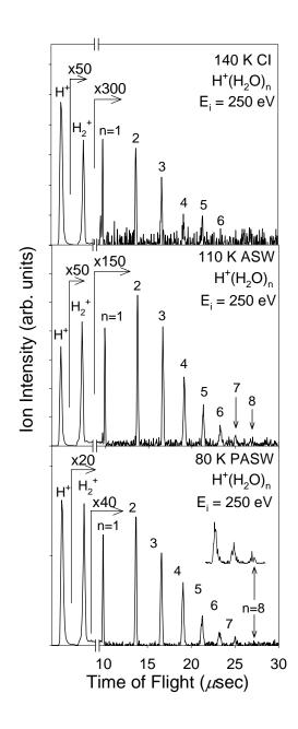
Figure 3.1 ESD-TOF from  $\sim 50$  ML of CI, ASW, and PASW
