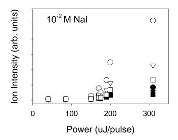
Figure 6.5 Power dependence of cation yield from a 10<sup>-2</sup> M NaI solution
