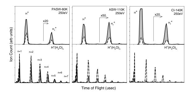
Figure 4.1 Cation yield of pristine and HCl dosed ice surfaces
