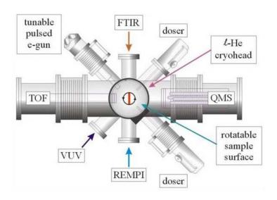
Figure 2.1 Schematic of UHV environmental surface science chamber
