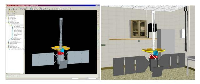
Figure 3: (a) CAD program view, and (b) full-scale VR view of a payload design.
