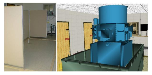
Figure 4: (a) Passive haptic objects in MiSL, and (b) the CALIPSO VE (including adapter).
