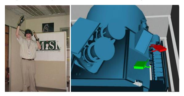
Figure 5: (a) A MiSL engineer attempts to reach the CALIPSO launch locks, and (b) the user's view.
