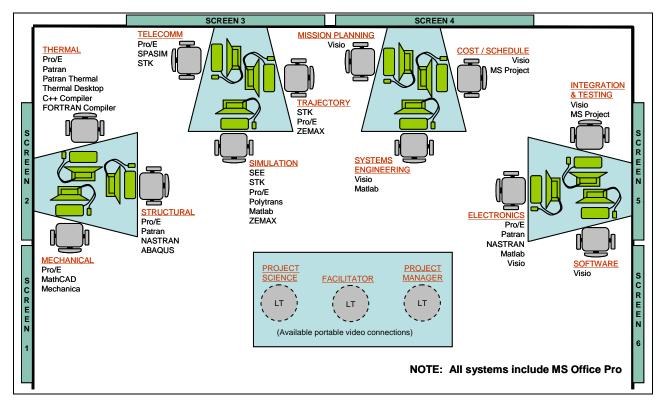
Figure 1: IDC layout showing typical discipline assignments.
